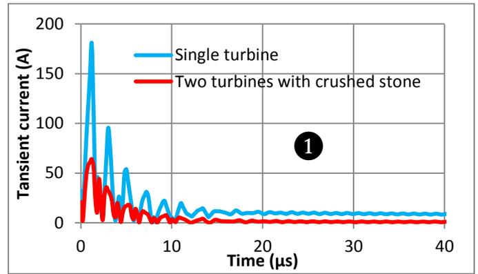
Figure 11. Current flowing through the body as a function of time – 10/350  $\mu$ s waveform
