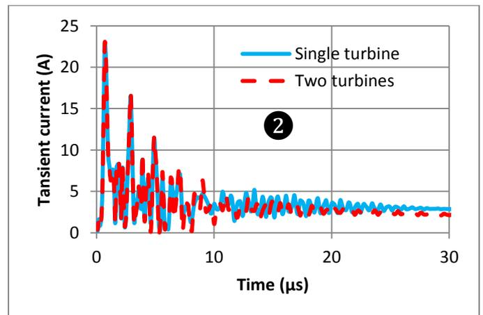
Figure 12. Current flowing through the legs as a function of time – 0,25/100  $\mu$ s waveform
