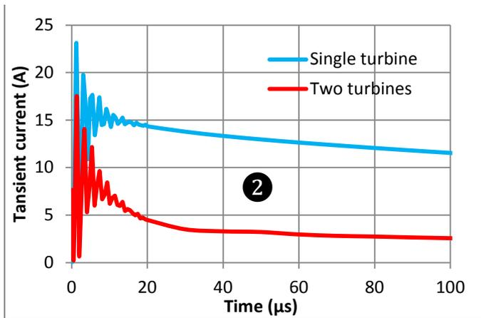
Figure 13. Current flowing through the legs as a function of time – 10/350  $\mu$ s waveform
