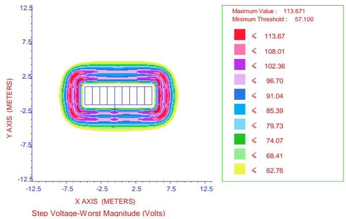
Figure 6. Step voltage distribution - HV fault
