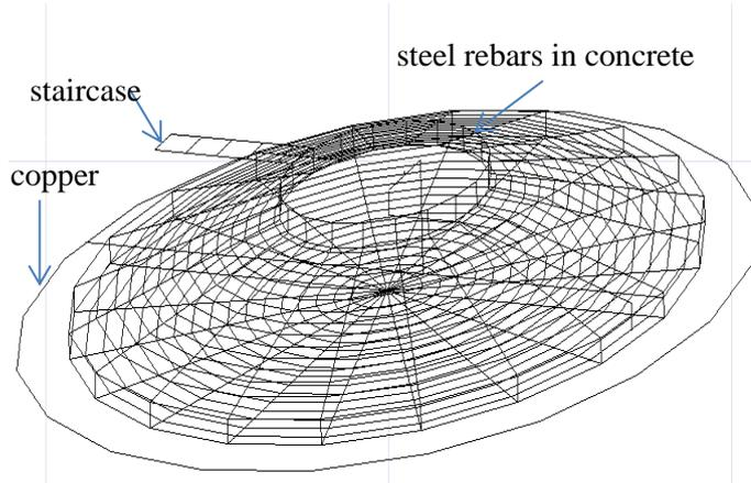
Figure 3. Perspective view of the wind turbine foundation model
