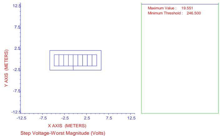
Figure 7. Step voltage distribution - MV fault
