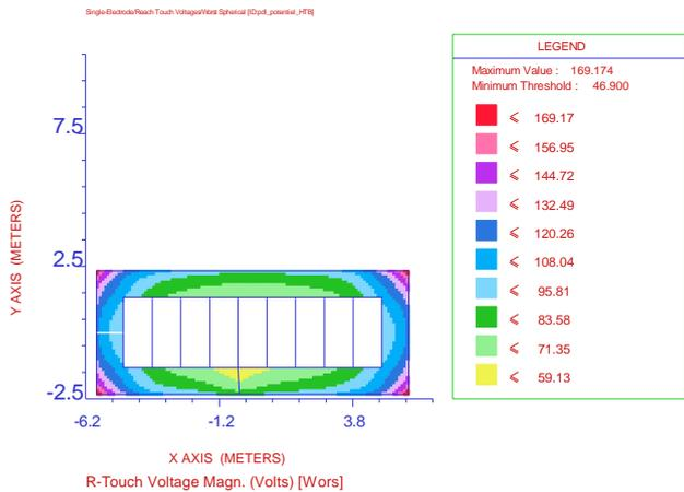
Figure 4. Touch voltage distribution - HV fault
