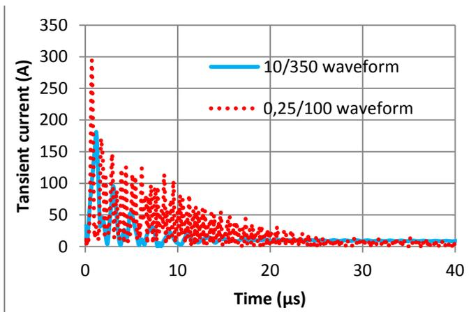
Figure 9. Current flowing through the body as a function of time
