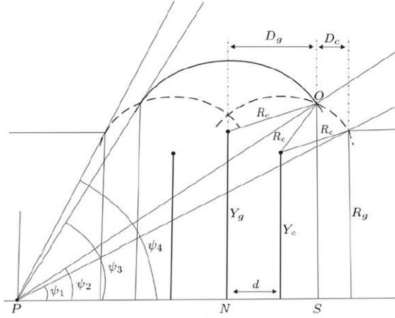
(a) Electro-geometric model of overhead line.
