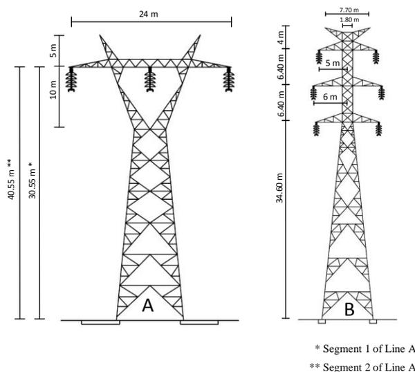
Figure 8. Transmission lines case study: A – 400 kV single circuit tower; B – 150 kV double circuit tower
