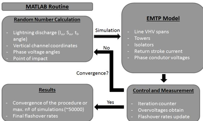
Figure 1. Interactions between tasks implemented for lightning flashover rate calculation
