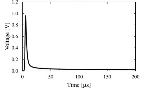
Fig. 3. Potential rise waveform (Size of foundation:  $20 \text{ m} \times 20 \text{ m}$ , grounding resistivity:  $1 \Omega\text{m}$ , wave front duration:  $2.74 \mu\text{s}$ ).
