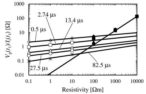
Fig. 7. Relation between  $V_p(t_i)/I_i(t_i)$  and grounding resistivity (Size of foundation:  $20 \text{ m} \times 20 \text{ m}$ )
