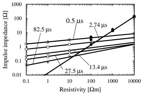
Fig. 5. Relation between impulse impedance and grounding resistivity (Size of foundation:  $20 \text{ m} \times 20 \text{ m}$ )
