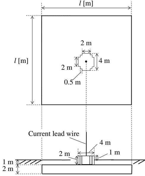
(a) Foundation model in the case of  $l \text{ m} \times l \text{ m}$
