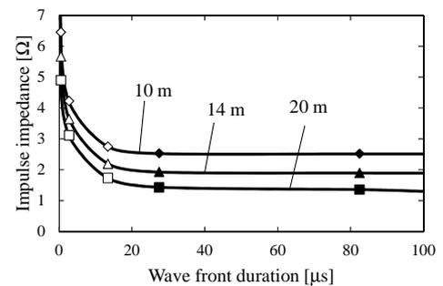
Fig. 8. Relation between impulse impedance and wave front duration (Size of foundation:  $10 \text{ m} \times 10 \text{ m}$ ,  $14 \text{ m} \times 14 \text{ m}$  and  $20 \text{ m} \times 20 \text{ m}$ , Grounding resistivity:  $100 \Omega\text{m}$ )
