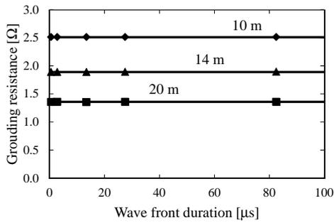
Fig. 9. Relation between grounding resistance and wave front duration (Size of foundation: 10 m × 10 m, 14 m × 14 m and 20 m × 20 m, Grounding resistivity: 100 Ωm)
