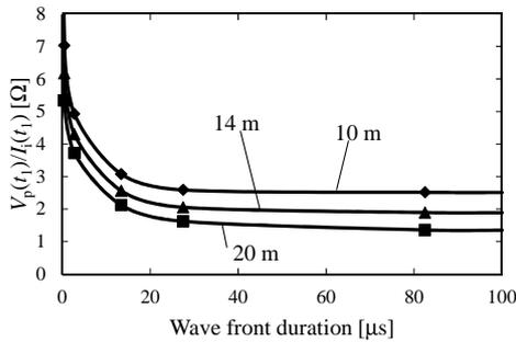
Fig. 10. Relation between values of  $V_p(t_f)/I_i(t_f)$  and wave front duration (Size of foundation: 10 m × 10 m, 14 m × 14 m and 20 m × 20 m, Grounding resistivity: 100 Ωm)
