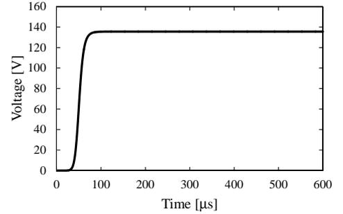
Fig. 4. Potential rise waveform (Size of foundation:  $20 \text{ m} \times 20 \text{ m}$ , grounding resistivity:  $1000 \Omega\text{m}$ , wave front duration:  $27.5 \mu\text{s}$ )
