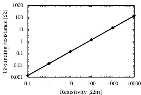
Fig. 6. Relation between grounding resistance and grounding resistivity (Size of foundation:  $20 \text{ m} \times 20 \text{ m}$ )
