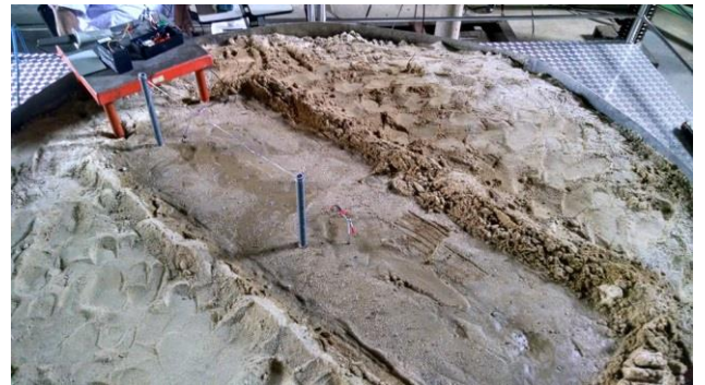
Figure 16. Photograph of the aerial line used to connect the ground electrodes.
