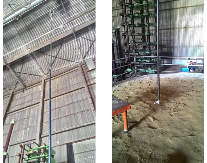
Figure 14. Photograph of the vertical transmission line used to simulate the lightning channel.
