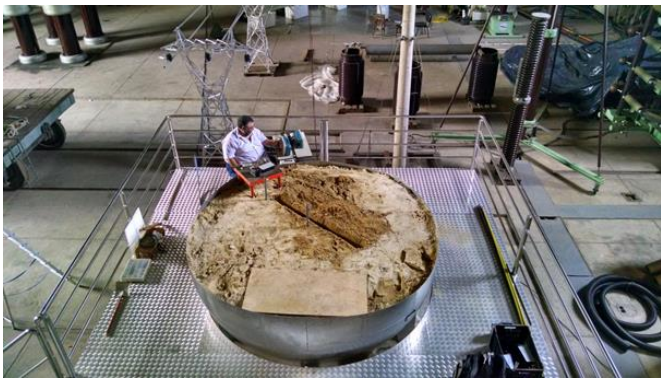
Figure 12. Hemispherical steel tank full of wet sand.
