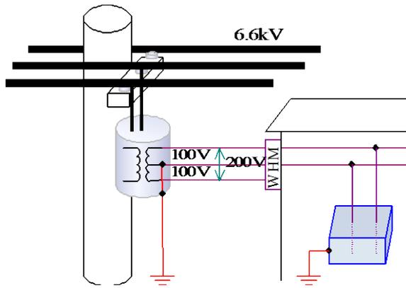
Figure 3. Japanese grounding system in the low-voltage circuit
