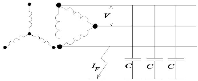
Figure 2. Japanese grounding system in the medium voltage circuit
