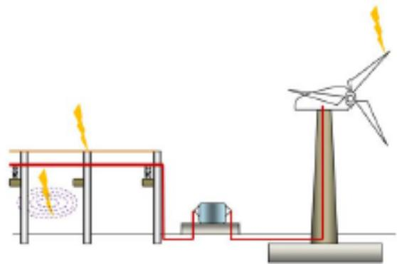
Figure 4. Lightning surges come into a wind turbine generation system
