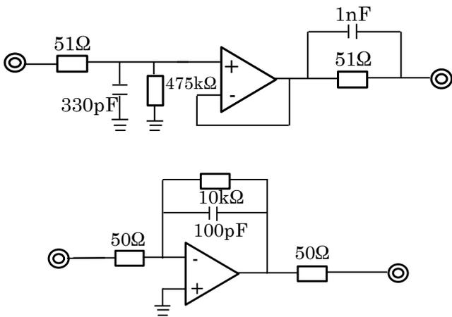
Figure 2. Top: Original circuit for the BOLT sensors with a 160  $\mu$ s time constant. Bottom: Redesigned DDT circuit with a 1  $\mu$ s time constant.
