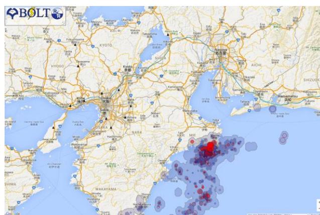
Figure 1. BOLT real-time display. Small black triangles indicate the location of sensor sites around the Kansai area of Japan. Lightning activity to the south-east of the network shows flash location, current, polarity, and extent density in an intuitive combined display.
