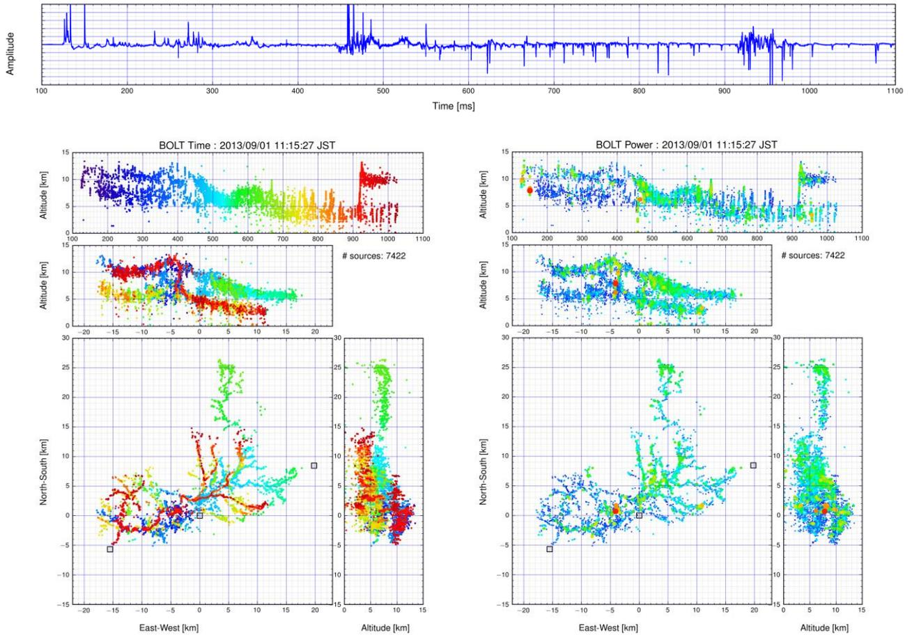
Figure 5. Example of improved BOLT mapping for a single IC flash. Top: time series electric field waveform record. Bottom: 3D maps of the LF lightning source locations colored by time (left) and estimated peak current (right). The 3D maps are shown in standard engineering format, displaying time-elevation, plan and vertical cross-sections.
