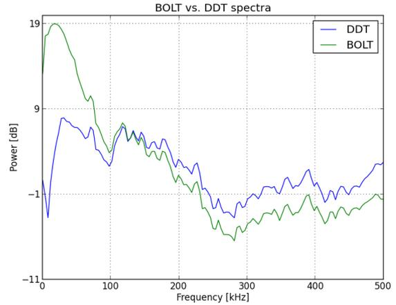
Figure 3. Frequency response of the original BOLT antenna, and the new DDT redesign. The new DDT antenna is less sensitive at frequencies lower than about 100 kHz, but more sensitive at frequencies above 100 kHz.
