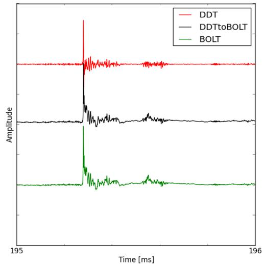
Figure 4. The time differentiated signal from the DDT circuit can be converted into the signal measured with the original BOLT antenna using a digital filter. The agreement between the digitally converted DDT and BOLT signals is excellent.
