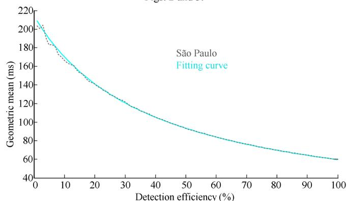
Figure 8. Geometric mean of the interstroke interval as a function of DE for interstroke intervals observed in São Paulo (in gray). A fitting curve is plotted in blue.
