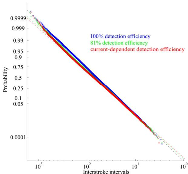
Figure 6. Cumulative probability distribution of interstroke intervals for Arizona and current-dependent detection efficiency (in red). Since this detection efficiency results in the removal of 19% of samples, it is compared with the cumulative probability for 81% uniform detection efficiency. The results show that there is no significant difference in the final cumulative probability distribution. The dataset size was  $1e5$  flashes.
