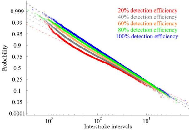
Figure 4. Cumulative probability distribution of interstroke intervals for São Paulo and detection efficiency ranging from 20% to 100%.
