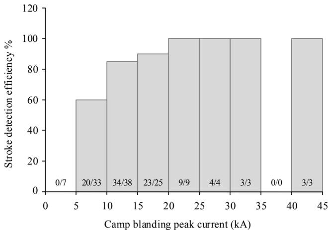
Figure 3. Stroke detection efficiency as a function of peak current. The ratio given inside each column represents the number of strokes detected by the lightning detection system over the number of strokes recorded directly. Adopted from [9].
