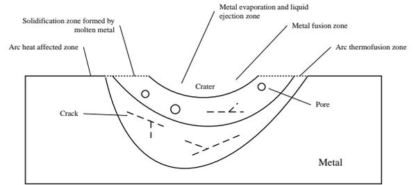
Figure 15. Schematic diagram of craters, pores and cracks created on metal under action of long stroke
