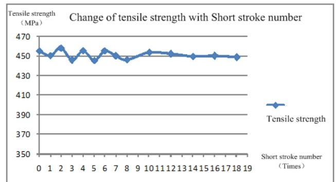
Figure 7. Short stroke test results
