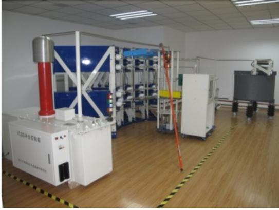
Figure 1. Impulse current generator
