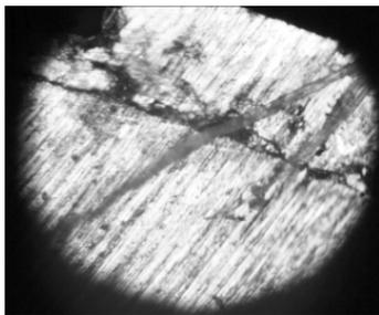
Figure 14. Cracks observed on cross section of lightning strike point at high-tensile steel wires ( $\Phi 8\text{mm}$ ) of bridge cable (under  $100\times$  magnification)
