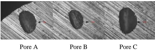
Figure 13. Pores created on cross section of lightning strike point (under  $100\times$  magnification)
