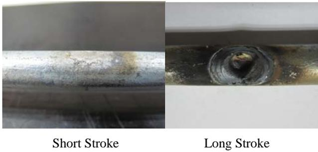
Figure 12. Comparison of damages occurred to galvanized round steel ( $\Phi 12\text{mm}$ ) surface under short stroke and long stroke
