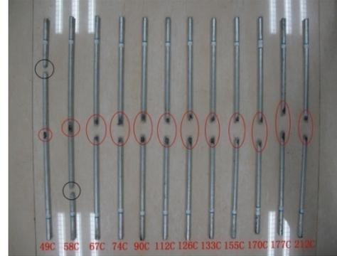
Figure 11. Breakpoints of tension test coincided with light strike points when electric discharges of long stroke added up to a certain level
