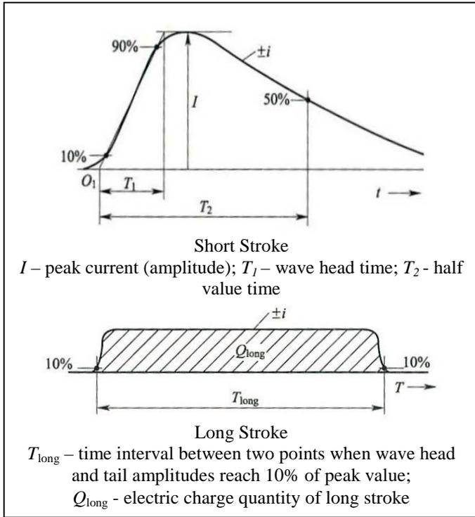
Figure 4. Short stroke (typical value  $T_2 < 2\text{ms}$ ) and long stroke (typical value  $2\text{ms} < T_{long} < 1\text{s}$ )
