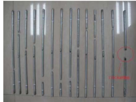
Figure 9. Comparison of tension test results following short stroke and long stroke
