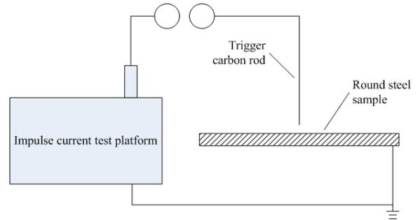
Figure 5. Schematic diagram of simulated lightning stroke test
