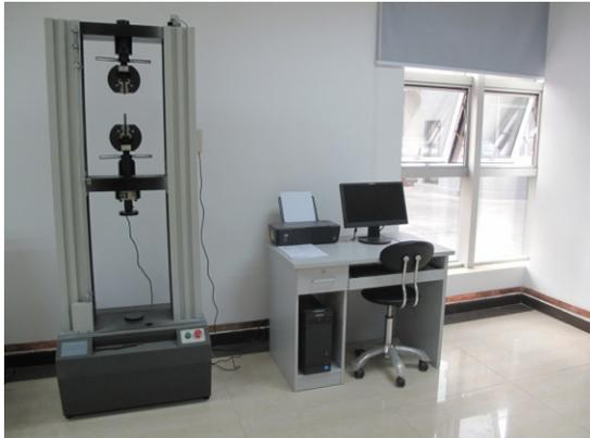
Figure 2. Electronic tension tester
