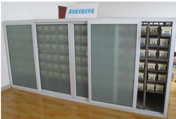
Figure 3. Sample case used in laboratory corrosion test
