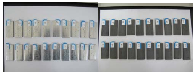
Figure 1. Galvanized and non-galvanized flat steels
