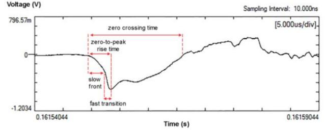
Figure 2. Definitions for the slow front duration, fast transition time, zero-to-peak rise time and zero crossing time
