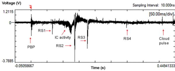
Figure 1. A four-stroke positive ground flash recorded in Sweden (Flash no.55 recorded on 7<sup>th</sup> August 2014 at 07:41:23378875)
