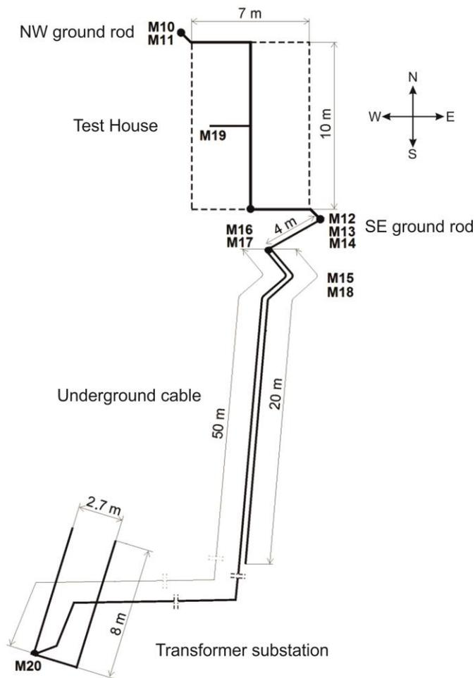
Figure 2. Schematic diagram of experimental setup and test object with measurement points M10-M20 described in the paper.
