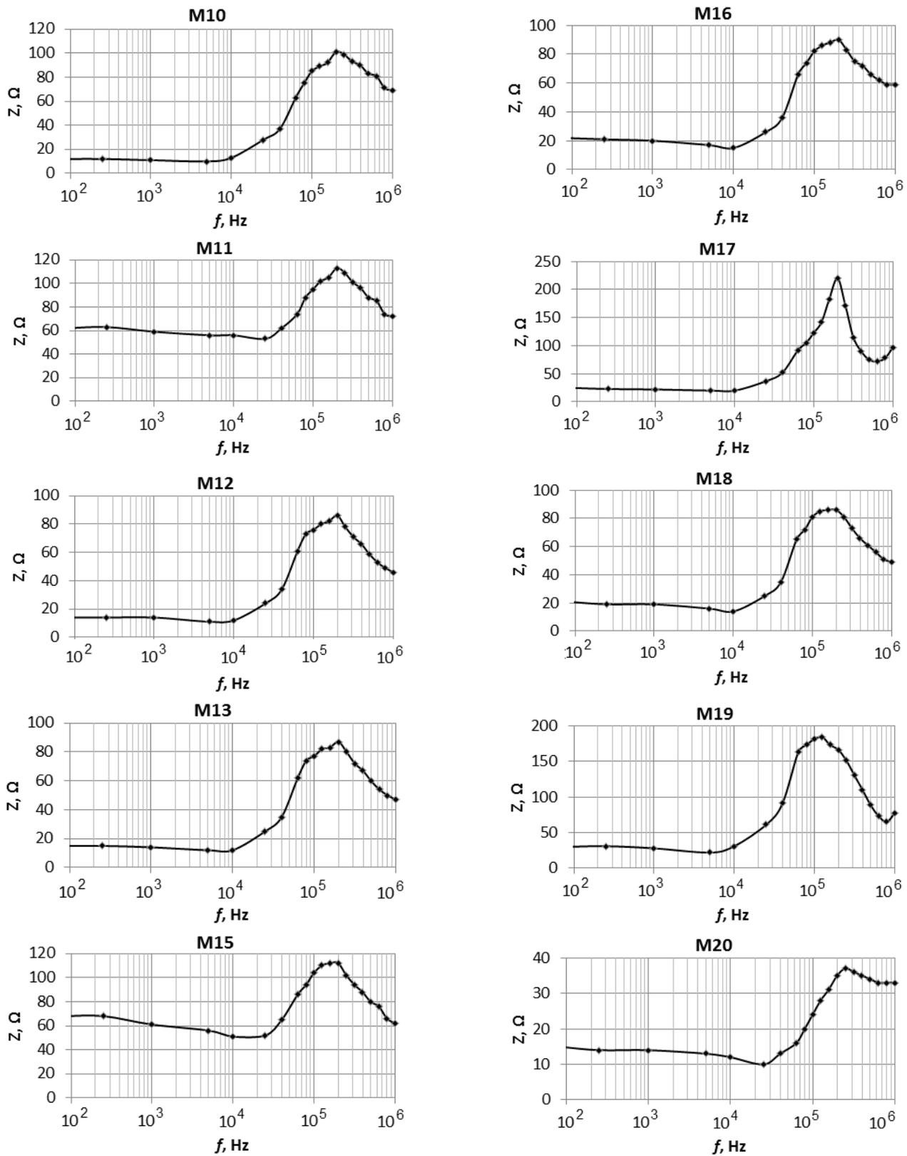
Figure 3. Frequency characteristics of grounding impedances measured at the test site in Huta Poreby during the summer season in 2015.
