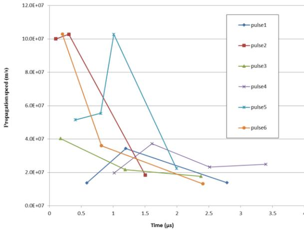
Figure 8. Leader pulse discharge propagation speed versus time.
