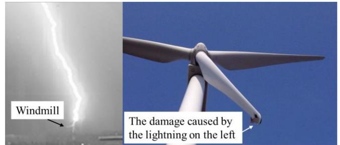
Figure 1. The picture of the lightning and the damage caused by this lightning.
