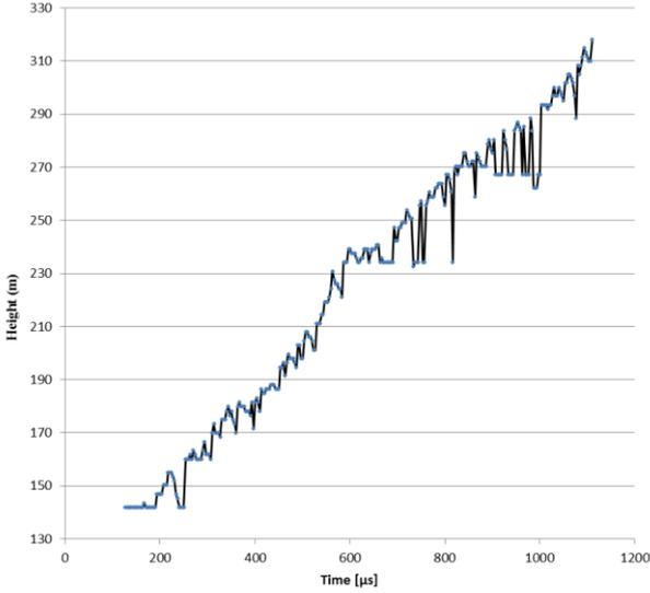
Figure 7. Height of the upward negative leader tip versus time.
