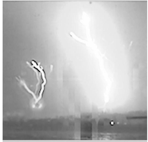
Figure 6. Photo of the upward negative connecting leader immediately prior to the return stroke type of discharge.
