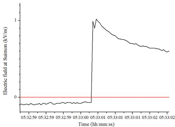
Figure 5. The electric field measured by a field mill at ground at a distance of about 400 m from the windmill.
