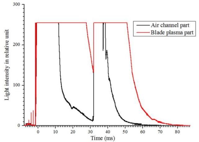
Figure 10. Luminosity waveforms of air channel part and the blade plasma part.
