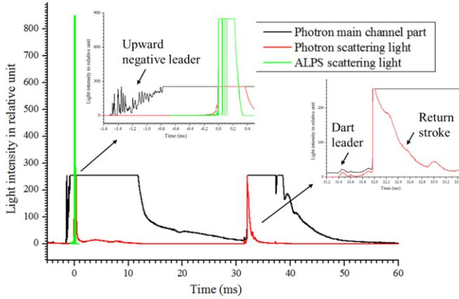
Figure 3. Luminosity waveforms of recorded by Photron camera and ALPS.
