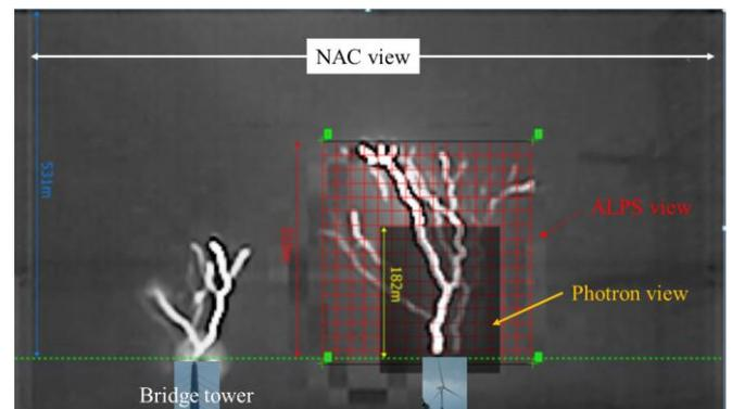
Figure 2. Views of the three high speed optical observation systems used in this study.
