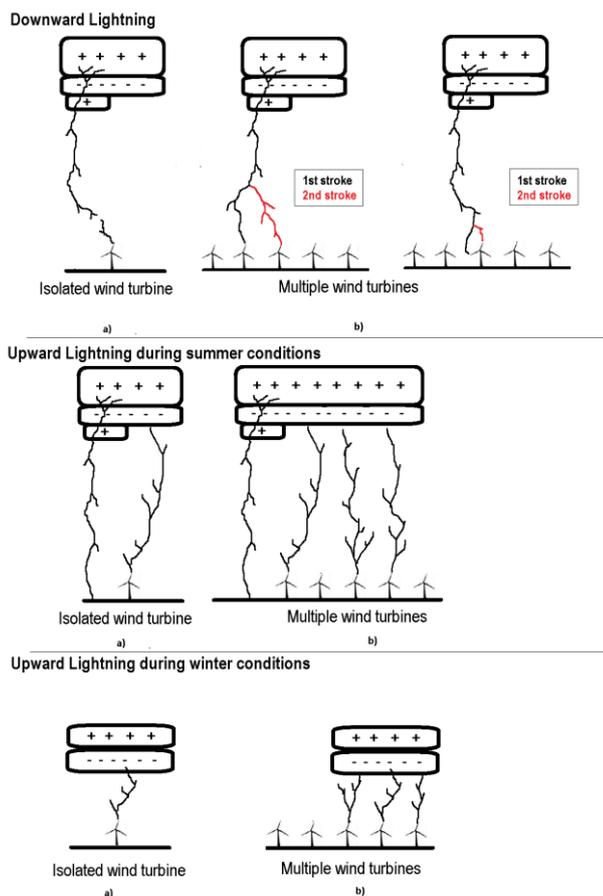
Figure 1. Situations in which multiple ground strike points on a group of wind turbines can occur.
