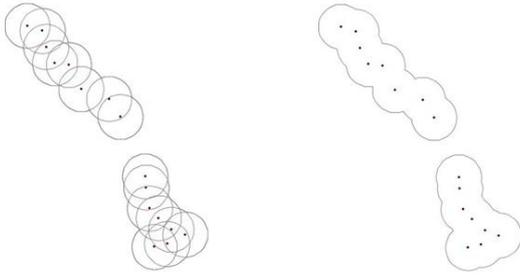
Figure 5. Collection area of a wind farm without overlapping and with overlapping (black points represent wind turbines).
