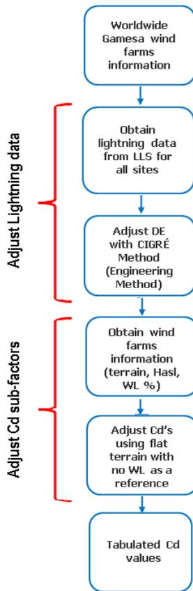
Figure 8. Flowchart to determine tabulated values for the environmental factors.
