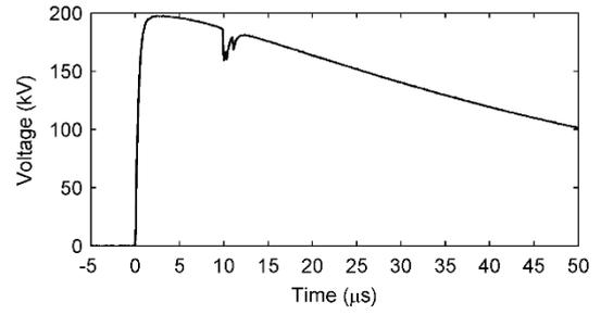
Figure 11. Voltage drop on the waveform measured during the occurrence of a partial disruptive discharge.
