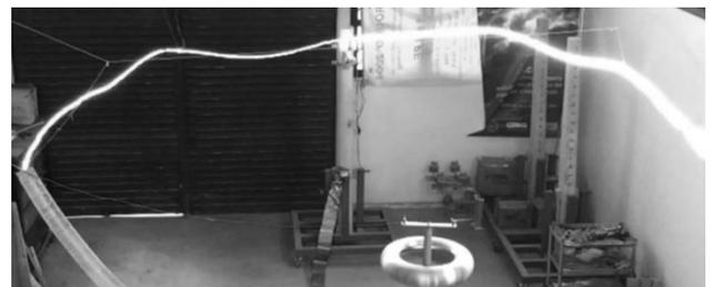
Figure 4. Surface discharge.
