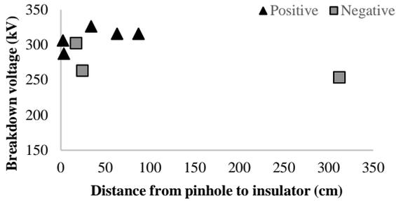
(b) Test without charge removal.
