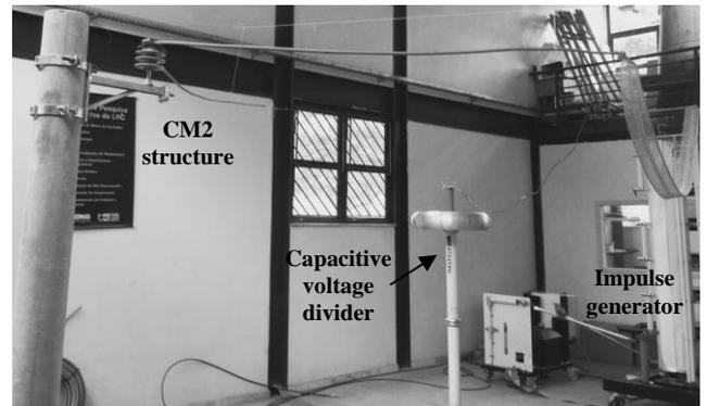
Figure 3. Experimental set-up at high voltage laboratory.
