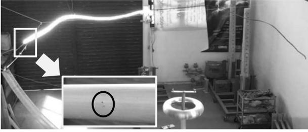
Figure 5. Disruptive discharge with pinhole formation in the XLPE-cover (or breakdown).
