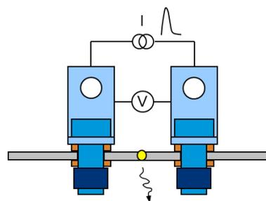
Figure 1. Test principles for preliminary edge glow characterization [1].
