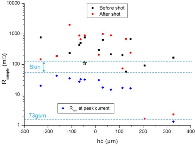
Figure 9. Sample resistance versus contact height of the fastener; ■ before the shot; ● after the shot; ◆ during the shot at peak current; ★ before arcing
