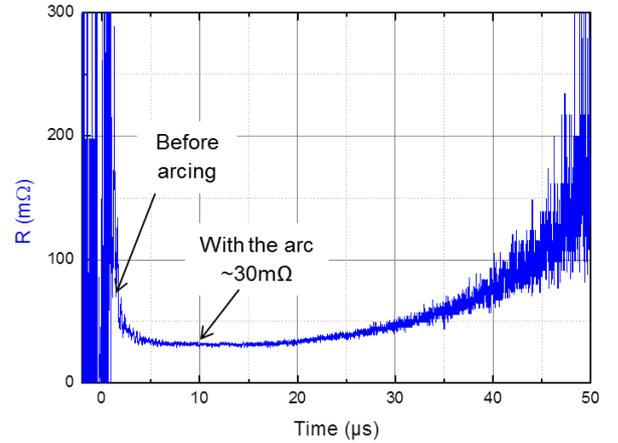
Figure 8. Sample resistance versus time for  $h_c = -45\mu\text{m}$ .
