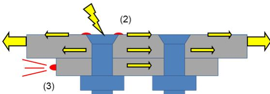
Figure 3. Current distribution at local assembly level.
