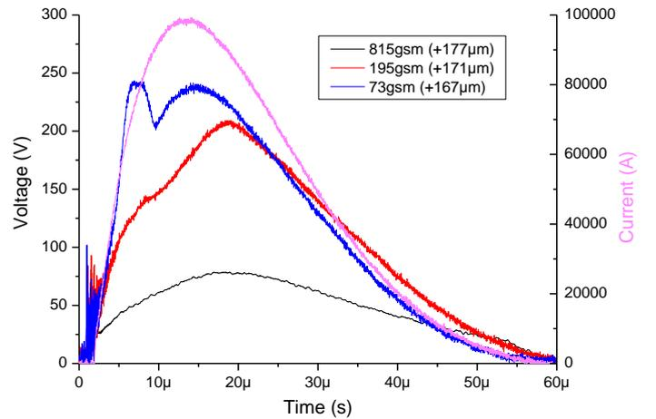
Figure 12. Current and voltage drop waveforms versus time for various lightning protection densities.
