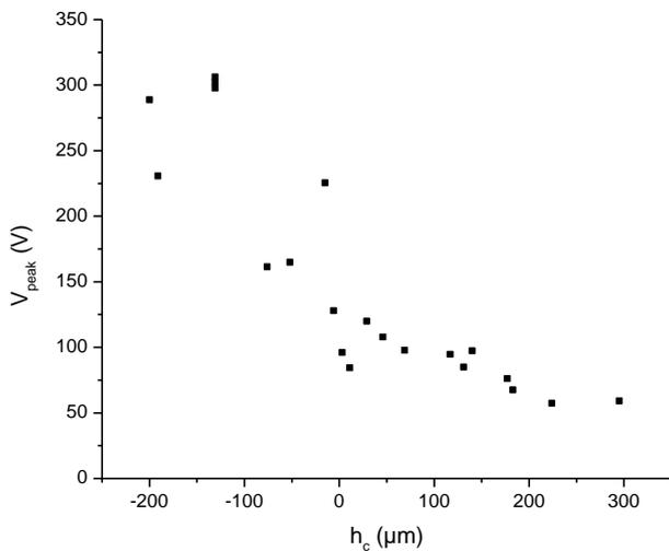
Figure 13. Peak voltage drop versus contact height of the fastener
