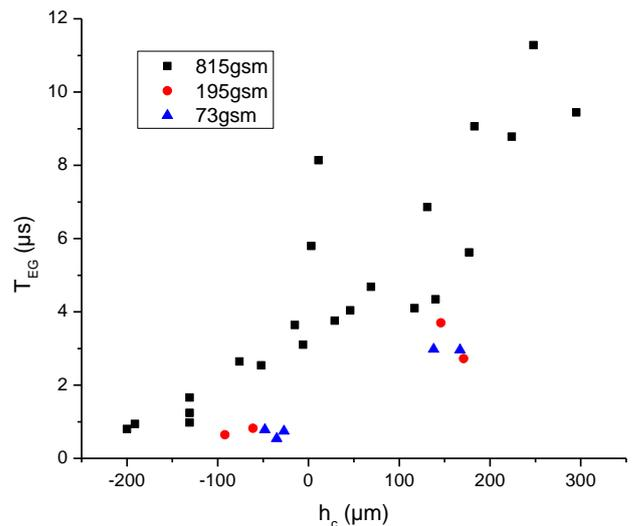
Figure 15. Edge glow apparition delay versus contact height of the fastener and for various lightning protection densities.
