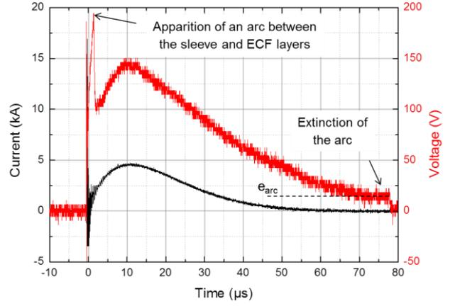
Figure 7. Current and voltage drop waveforms versus time for  $h_c = -45\mu\text{m}$ .
