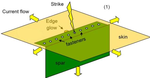
Figure 2. Current distribution at global assembly level.
