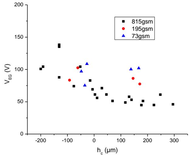
Figure 14. Voltage drop threshold for edge glow occurrence versus contact height of the fastener and for various lightning protection densities.
