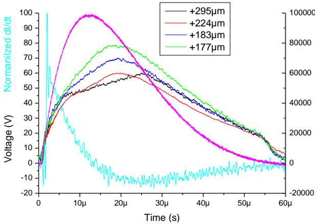
Figure 10. Current and voltage drop waveforms versus time for  $h_c > 170\mu\text{m}$
