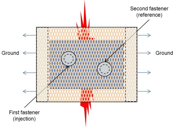
Figure 6. Assembly test coupons for edge glow analysis
