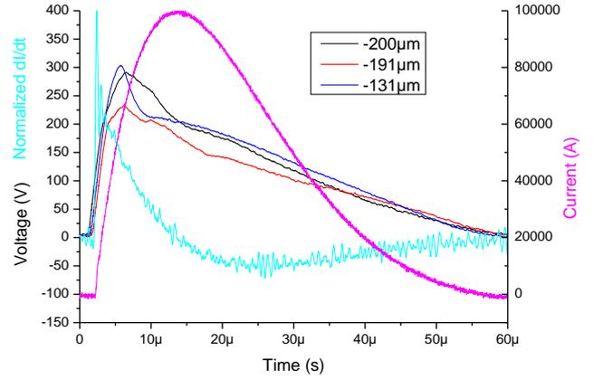
Figure 11. Current and voltage drop waveforms versus time for  $h_c < -130\mu\text{m}$
