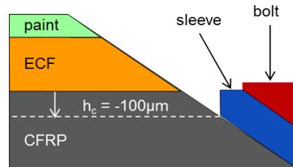
Figure 5. Contact height ( $h_c$ ) of fastener with respect to bottom ECF layer.
