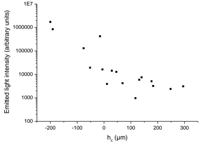
Figure 17. Emitted light intensity versus contact height of the fastener.
