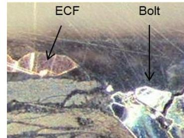
Figure 4. Micro-cut of the contact area between bolt and lightning protection
