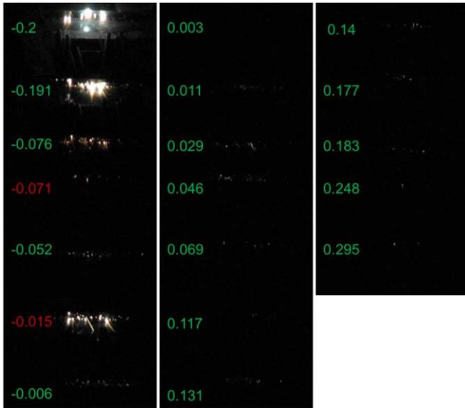
Figure 16. Still camera pictures, capturing the edge glow emission during shot, versus contact height of the fastener (indicated on each figure in mm).
