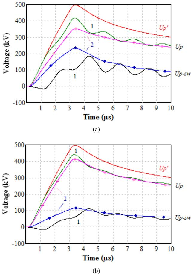
Figure 4. Lightning-induced voltages  $Up'$ ,  $Up$ , and  $Up-sw$  at the point closest to the stroke location.  $I = 50 \text{ kA}$ ;  $t_f = 3 \mu\text{s}$ ;  $v_f = 0.3 \text{ c}$ ;  $d = 50 \text{ m}$ ;  $h = 10 \text{ m}$ ;  $hg = 11 \text{ m}$ ;  $xg = 300 \text{ m}$ ;  $\rho = 1000 \Omega\text{m}$ .
