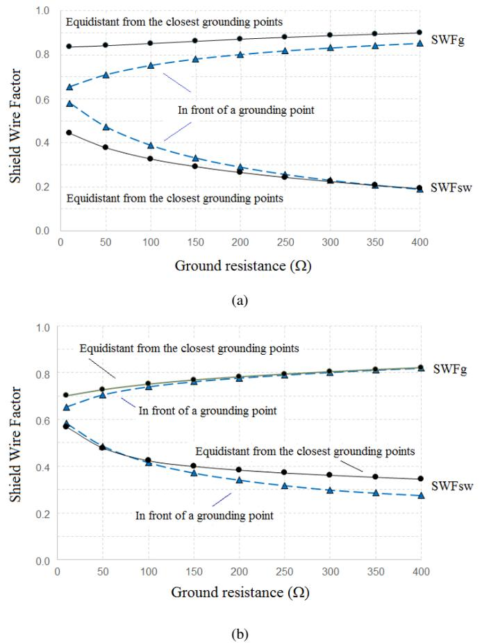
Figure 3. Shield wire factors at the point of the line closest to the stroke location as function of the ground resistance  $R_g$ , for two different positions of the stroke location in relation to the closest grounding point.  $I = 50$  kA;  $t_f = 3 \mu\text{s}$ ;  $v_f = 0.3 c$ ;  $h = 10$  m;  $h_g = 11$  m;  $x_g = 300$  m;  $R_g = 50 \Omega$ ;  $\rho = 1000 \Omega\text{m}$ . a)  $d = 50$  m b)  $d = 200$  m
