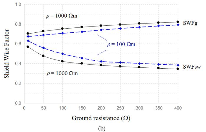
Figure 2. Shield wire factors  $SWF_g$  and  $SWF_{sw}$  at the point of the line closest to the stroke location as function of the ground resistance  $R_g$  for two values of the soil resistivity.  $I = 50$  kA;  $t_f = 3$   $\mu$ s;  $v_f = 0.3 c$ ;  $h = 10$  m;  $hg = 11$  m;  $xg = 300$  m;  $R_g = 50$   $\Omega$ ; stroke location equidistant from the closest grounding points. a)  $d = 50$  m b)  $d = 200$  m
