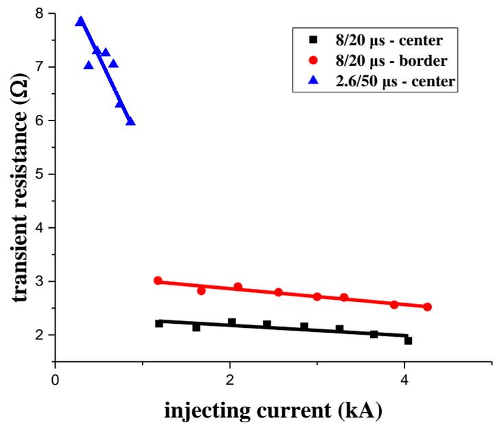
Figure 4. Transient resistance with different current amplitudes
