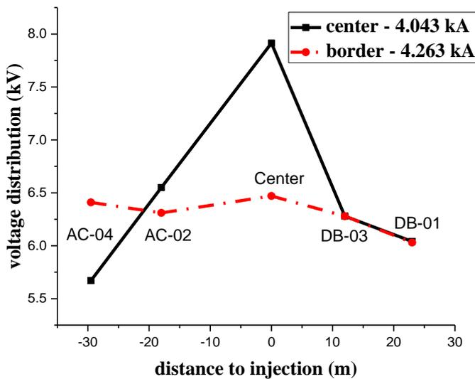
Figure 5. Voltage distribution of horizontal observations with different injecting position
