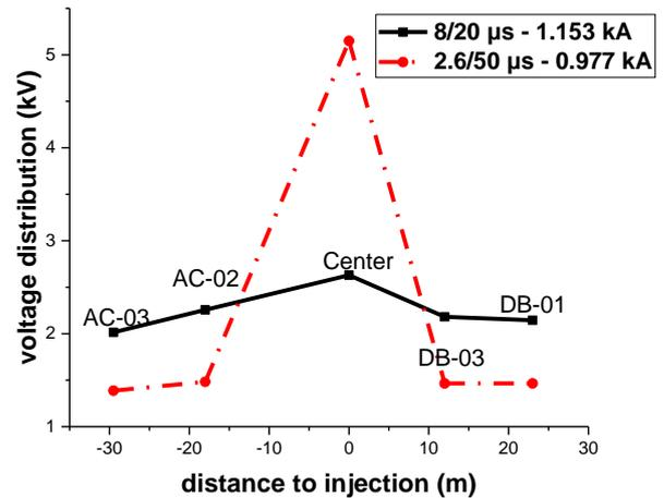
Figure 6. Voltage distribution of horizontal observations with different injecting position
