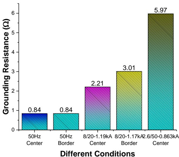
Figure 8. Grounding resistances comparison
