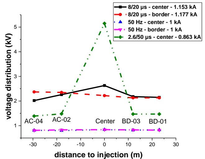
Figure 9. Voltage distribution of conductors on horizontal observations
