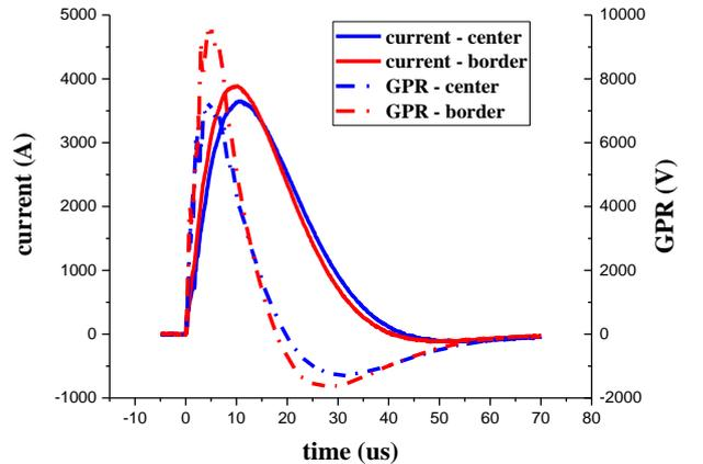
Figure 2. Injecting current and grid GRP with different injecting positions
