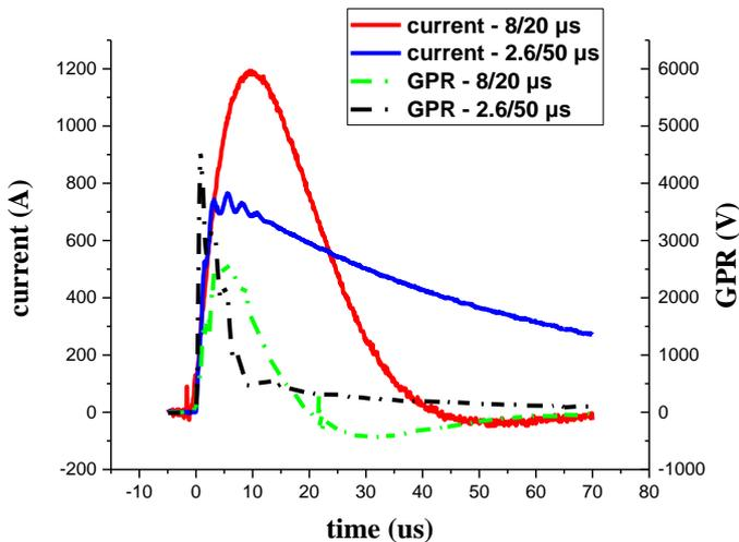
Figure 3. Injecting current and grid GRP with different waveforms
