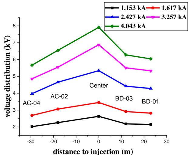
Figure 7. Voltage distribution of horizontal observations with different injecting amplitudes
