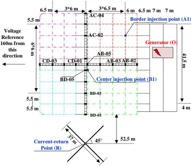
Figure 1. Simplified layout of the testing field
