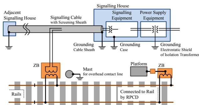
Figure 1 Grounding configuration of wayside equipment and constructions along Shinkansen tracks.
