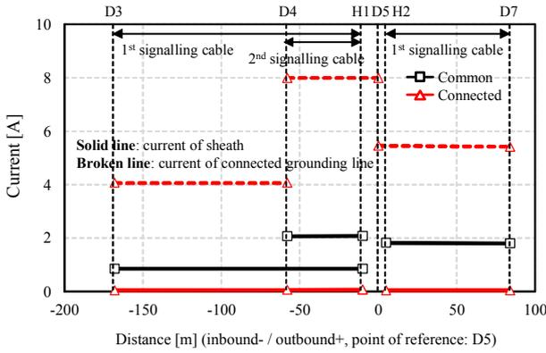
Figure 9 Shunt current at each measuring point (ground fault).
