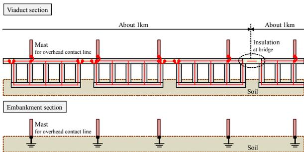
Figure 4 Schematic illustration of grounding systems on track structure.
