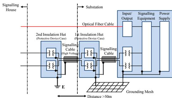
Figure 3 Schematic illustration of groundings in insulation hut and substation.
