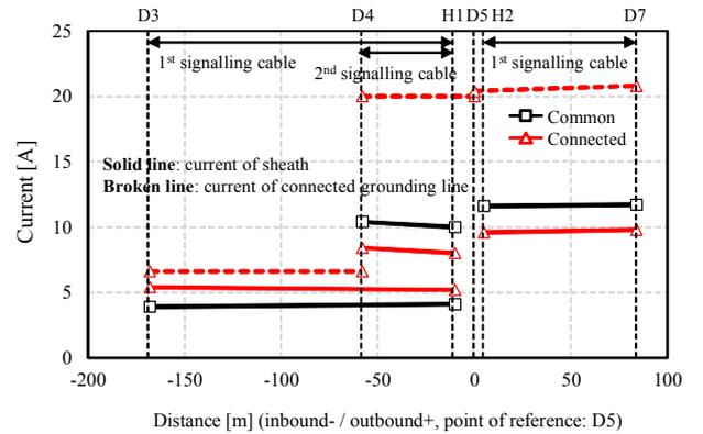
Figure 11 Shunt current at each measuring point (lightning surge).
