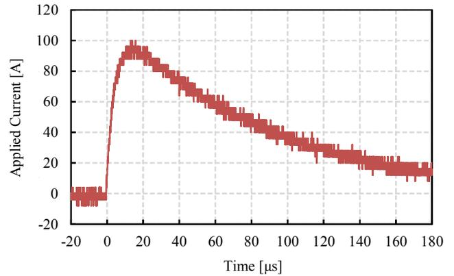
Figure 7 Waveform of applied current simulated lightning surge.
