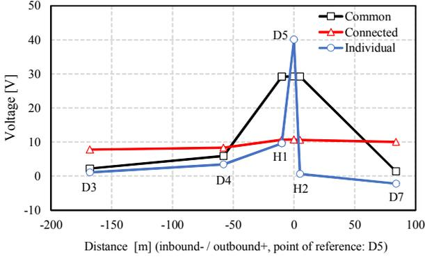
Figure 8 Voltage of groundings at each measuring point (ground fault).
