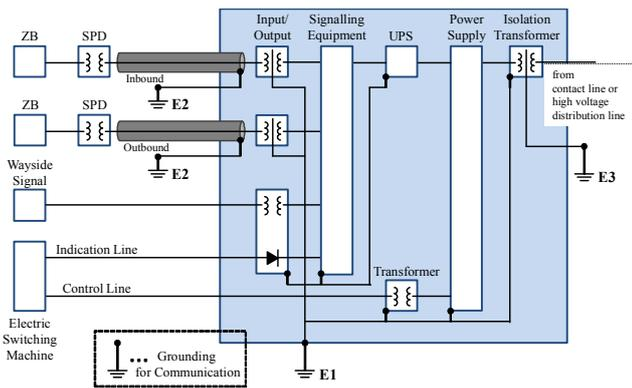
Figure 2 Schematic illustration of groundings in signalling house.
