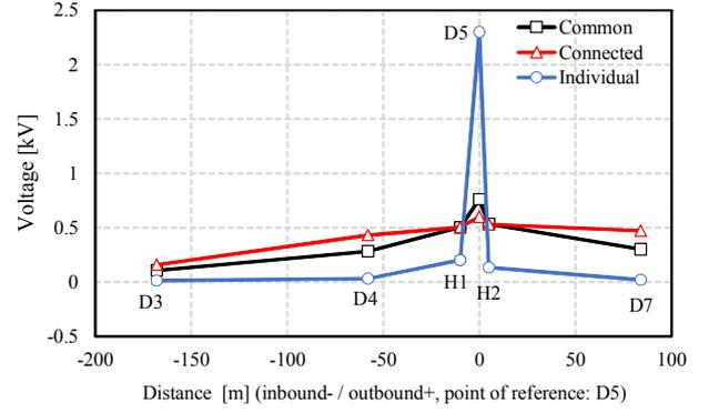
Figure 10 Voltage of groundings at each measuring point (lightning surge).
