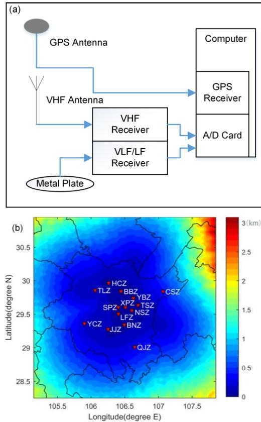
Figure 1 (a) hardware constitution of DULLS, (b) layout of the sensor network and vertical estimated errors at the altitude of 7 km given by a Monte Carlo simulations
