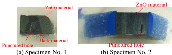
Figure 7. The cross sections of the punctured pieces
