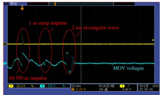
Figure 5. The degraded voltage waveforms on V275 under MODT
