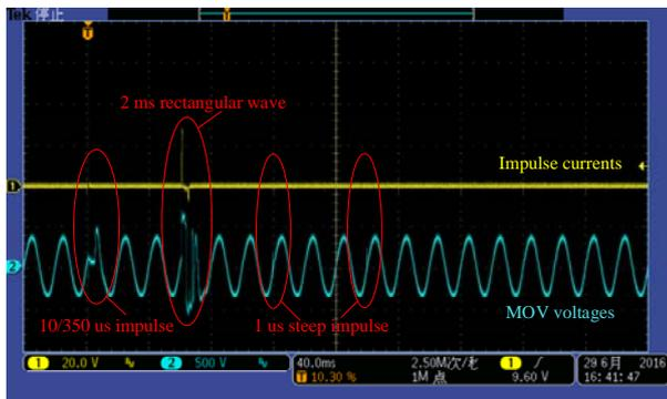
Figure 6. Current and voltage waveforms on V460 under 60 ms interval
