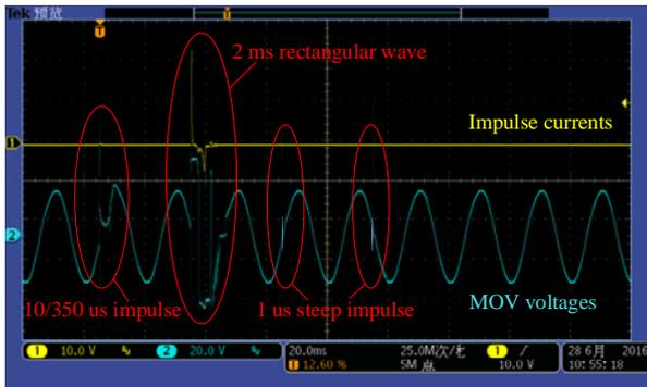
Figure 4. The current and voltage waveforms on V230 under MODT
