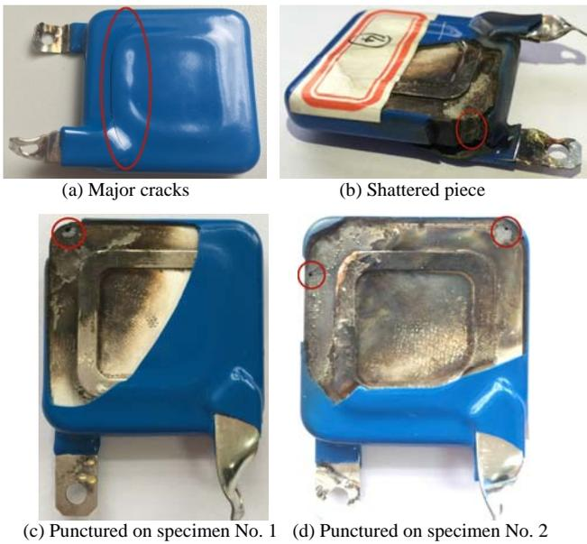
Figure 3. Main failure modes appear on varistors
