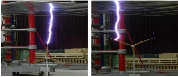
Figure 7. Representative photos taken by the cameras during the simulated upward lightning attachment test.
