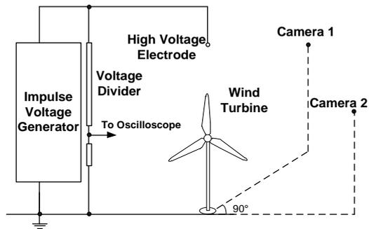
Figure 4. Experiment test system
