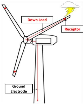
Figure 1. Schematic diagram of the lightning protection system of wind turbine generator
