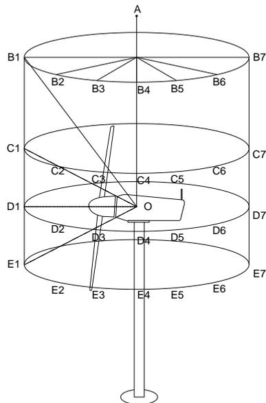
Figure 5. Position of the high voltage electrode
