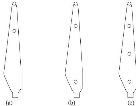
Figure 3. Layout of blade receptors with (a) two, (b) three, and (c) four pairs of receptors.
