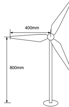
Figure 2. Structure size of the wind turbine model
