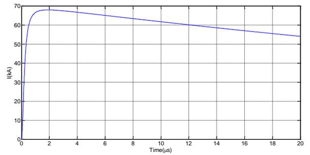
**Figure 4. The applied return stroke current wave shape for evaluation of lightning induced voltage on typical distribution line**
