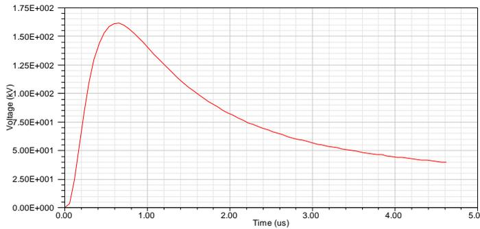
**Figure 3. Applied impulse voltage wave shapes (case a: standard wave shape, case b: lightning induced voltage wave shape)**
