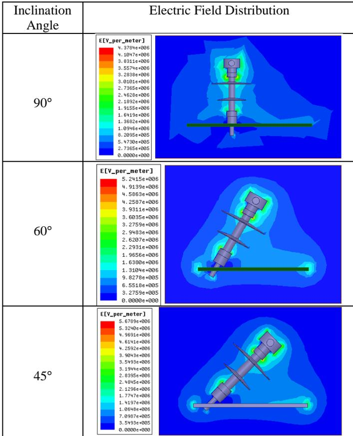
Figure.7. Electric field profiles under different angles for case a
