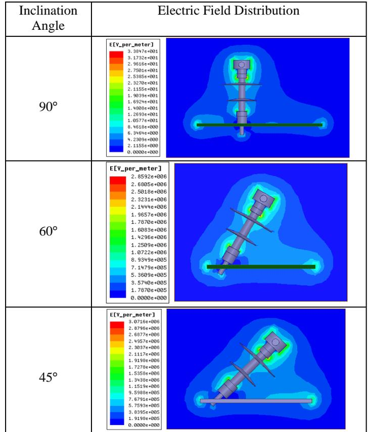
Figure.8 Electrical field profiles under different angles for case b
