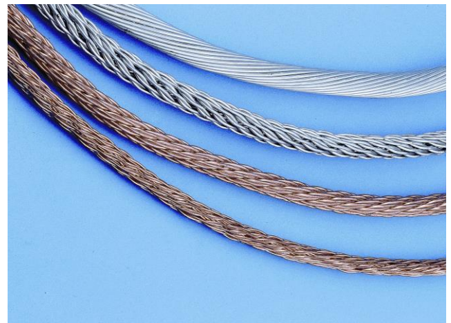
Figure 1. Typical conductor strands used in United States. Upper – Class II aluminum concentric strand; 2 nd – Class I aluminum smooth weave; 3 rd – Class II copper rope lay; Lower – Class I copper smooth weave.
