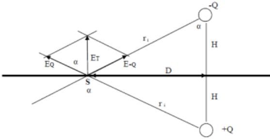
Figure 1: Image Method for Charge Transfer (adapted from [7])
