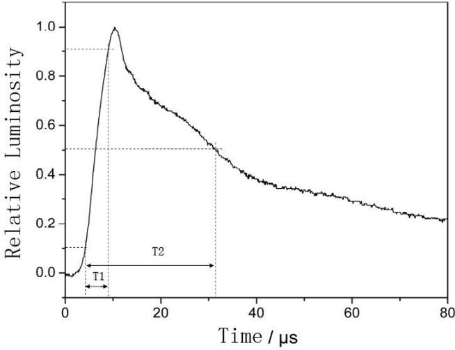
Figure 6 Illustration for the waveform parameters of luminosity pulse induced by lightning return stroke
