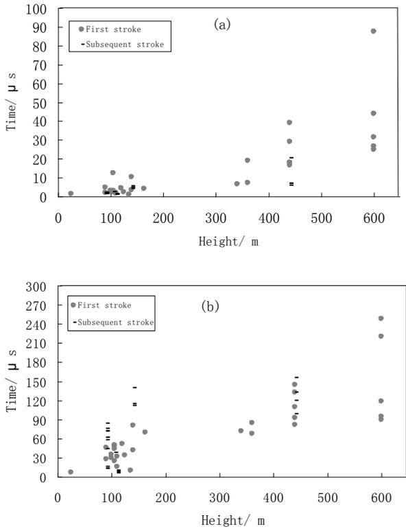
Figure 7 The  $T_1$  (a) and the  $T_2$  (b) of the luminosity pulses waveform induced by the return strokes versus the heights of the grounding points.
