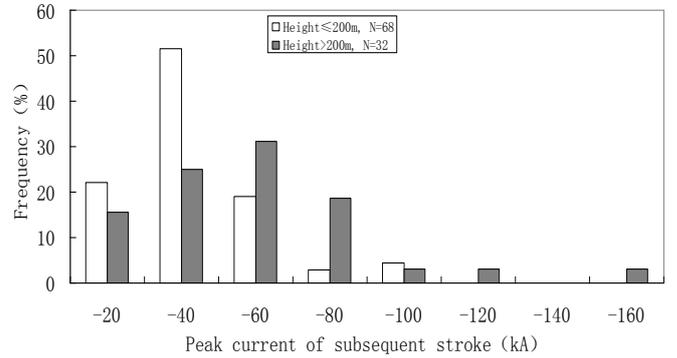
Figure 5 Distribution of  $I_{peak}$  for the subsequent strokes
