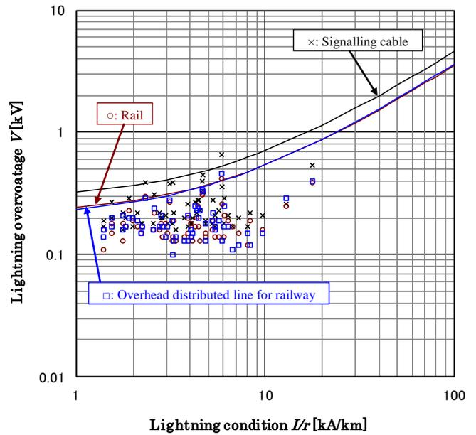
Figure 7. Correlation between lightning overvoltages and lightning conditions (electrified section).
