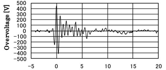
(a) Lightning overvoltages of SVV cable (“White” core).
