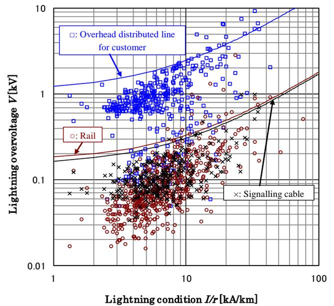
Figure 8. Correlation between lightning overvoltages and lightning conditions (non-electrified section).
