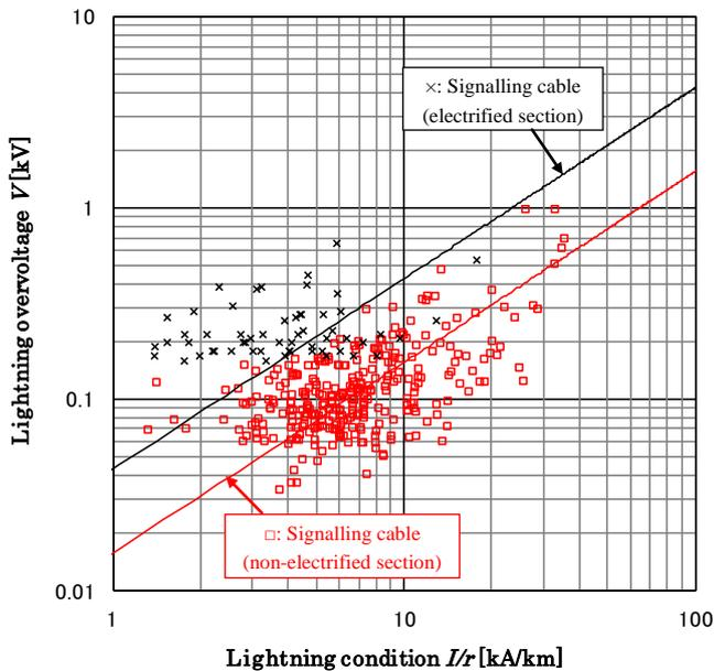
Figure 9. Comparison of the correlation between lightning overvoltages of signalling cables and lightning conditions in the electrified section with that in the non-electrified section.
