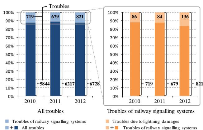
Figure 1. Troubles of railway signalling systems due to lightning damages.
