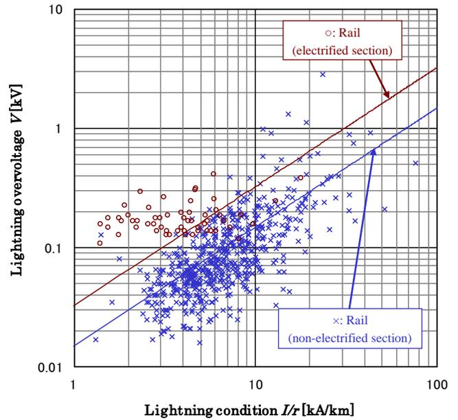
Figure 10. Comparison of the correlation between lightning overvoltages of rails and lightning conditions in the electrified section with that in the non-electrified section.
