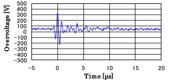
(c) Lightning overvoltages of overhead distributed line.
