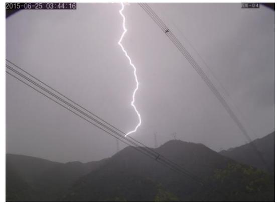
Figure.6 A ground flash stroke on 500kV transmission line
