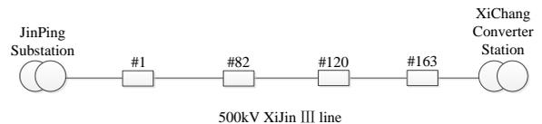
Figure.8 Terminal of the Transmission Line Distributed Fault Diagnosis System installation
