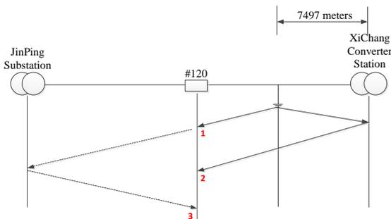
Figure.10 Positioning method schematic of the Transmission Line Distributed Fault Diagnosis System(1: Lightning traveling wave entering terminal no.120 from lightning strike point.2: Lightning traveling wave through the XiChang Converter Station reflected entering terminal no.120 again. 3: The lightning wave passed through the terminal no.120 firstly and then it was detected by the terminal no.120 again after reflected by the JinPing Substation)
