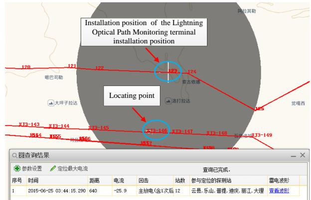
Figure.7 Locating results from Lightning Location System of the State Grid in China
