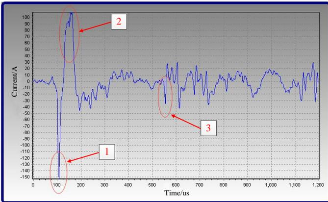
Figure.9 Lightning traveling wave record by terminal of the Transmission Line Distributed Fault Diagnosis System installed on no.120 tower C Phase(1: Lightning traveling wave entering terminal no.120 from lightning strike point.2: Lightning traveling wave through the XiChang Converter Station reflected entering terminal no.120 again. 3: The lightning wave passed through the terminal no.120 firstly and then it was detected by the terminal no.120 again after reflected by the JinPing Substation)
