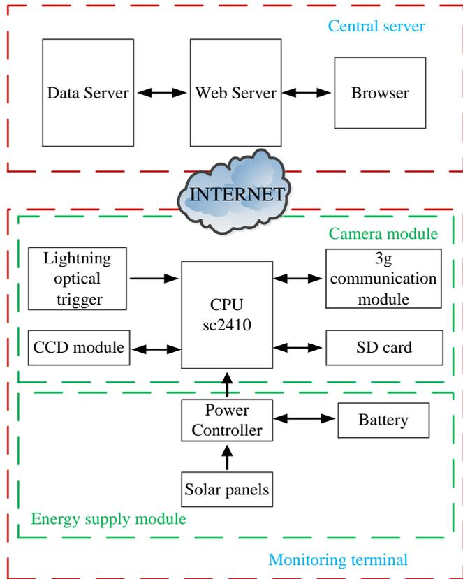
Figure. 1 System Diagram of the Lightning Optical Path Monitoring System
