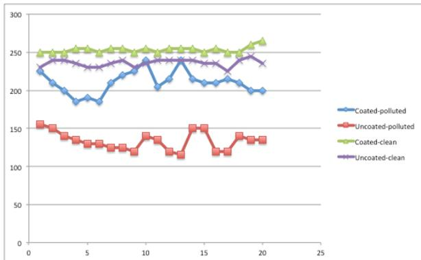
Figure 3. Comparison of Voltage Breakdown Values of a 10 kV polymer insulator (coated and uncoated) under Clean and Pollution (Salt) Conditions
