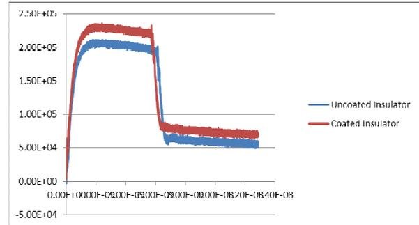
Figure 4. Voltage Breakdown Waveform for Insulator with Coating and without Coating under Wet Clean Conditions
