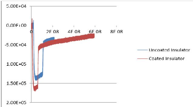
Figure 7. Voltage Breakdown Waveform for the Insulator with Coating and without Coating under Pollution (Salt) Conditions
