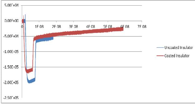
Figure 6. Voltage Breakdown Waveform for the Insulator with Coating and without Coating under Wet Clean Conditions
