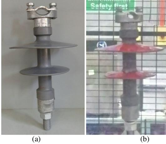
Figure 1. (a) 10 kV Polymer Insulator (b) 10 kV Polymer Insulator with Coating
