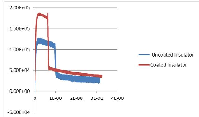
Figure 5. Voltage Breakdown Waveform for Insulator with Coating and without Coating under Pollution (Salt) Conditions
