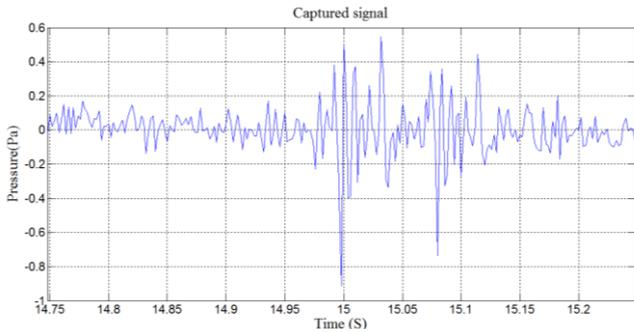
Figure 7. The pressure variation of two consecutive claps or a relection been captured from the thunder recorded as 04172014\_081013\_PM
