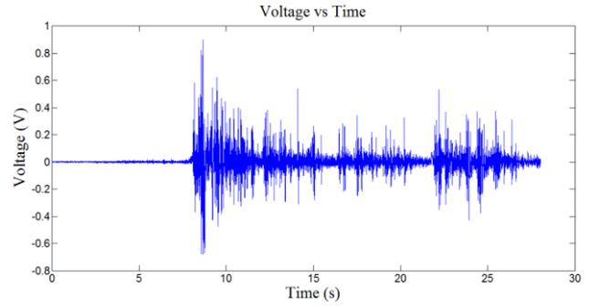
Figure 1. Recorded voltage variation of cloud flash (05092015\_030131\_PM)
