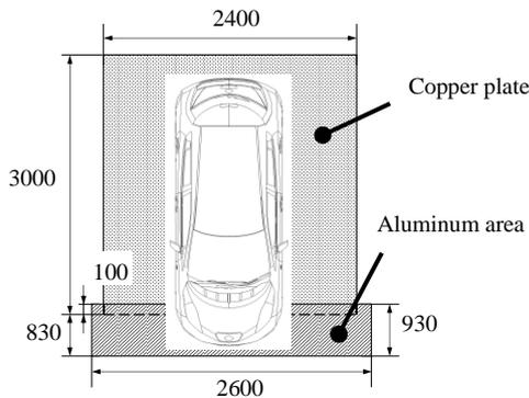
Figure 3. Dimensions of copper plate and expanded aluminum area.
