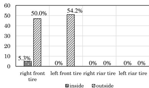
Figure 11. Number of creeping discharges on each wheel in discharge path verification test. (Charge voltage -200 kV)
