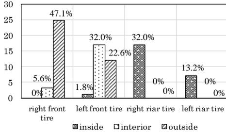
Figure 7. Number of creeping discharges on each wheel in discharge path verification test.
