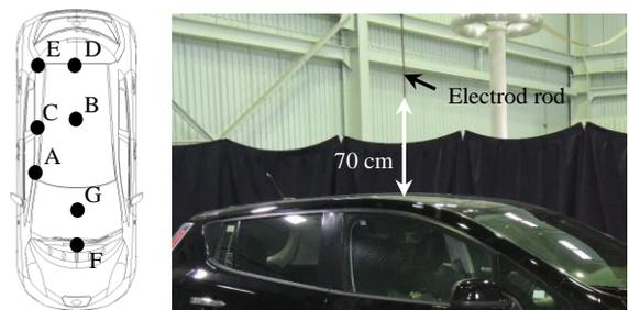
Figure 4. Placements of rod electrodes and its example.
