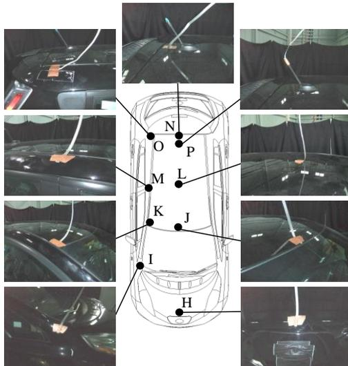
Figure 6. Connections of voltage-application points.
