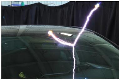
Figure 9. Creeping discharge of the front glass.
