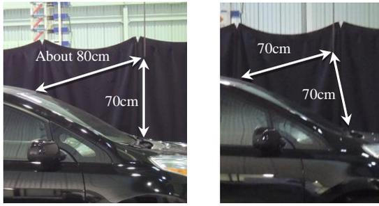
(a) 70 cm above the wiper (b) 70 cm above the wiper and roof
