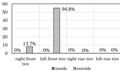
Figure 12. Number of creeping discharges on each wheel in discharge path verification test. (Charge voltage -500 kV)
