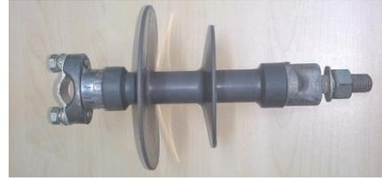
Fig. 1. A real 10 kV polymer insulator
