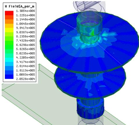
Fig. 9. Magnetic Field plot on insulator sheds for case B
