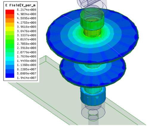
Fig. 7. Electric Field plot on insulator sheds for case B
