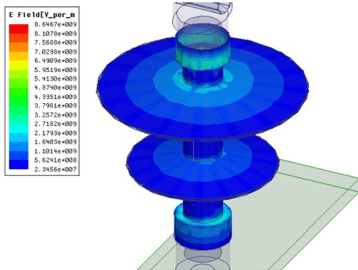
Fig. 6. Electric Field plot on insulator sheds for case A
