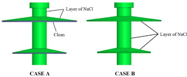
Fig. 3. Formation of pollution of Case A and Case B, partially and fully polluted insulator.
