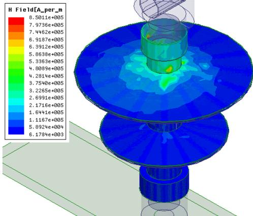
Fig. 8. Magnetic Field plot on insulator sheds for Case A
