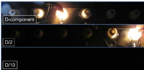
Figure 8. Photographs taken during scaled D-component strikes (Full D-component – top, D/2 – middle, D/10 – bottom)
