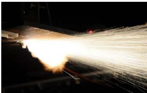
Figure 1. Open shutter photograph of an intense out-gassing event taken during an LDE test
