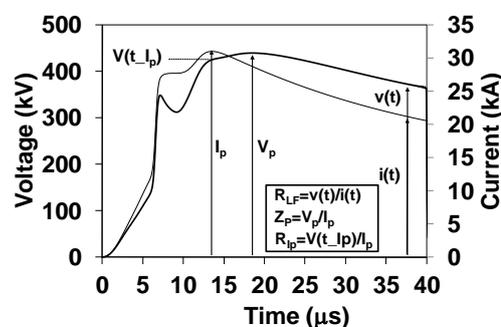
Figure 1. Response of counterpoise wires 70-m long buried 0.5 m deep in a 2000-Ωm soil subjected to a representative first-stroke lightning current, along with their concise representations  $Z_P$  and  $R_{LF}$ . Calculated  $Z_P$ ,  $R_{LF}$  and  $R_{IP}$ : 14.2 Ω, 18.9 Ω, and 13.7 Ω.
