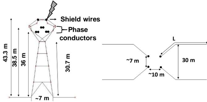
Figure 4. Representation of the tower configurations of the 230-kV line (a) and the tower-footing arrangement consisting of four counterpoise-wires (radius 0.75 cm) of length  $L$  buried 0.5 m deep in soil and 3-m long vertical rods (radius 5 cm) to represent the buried metallic components of the tower foundations.
