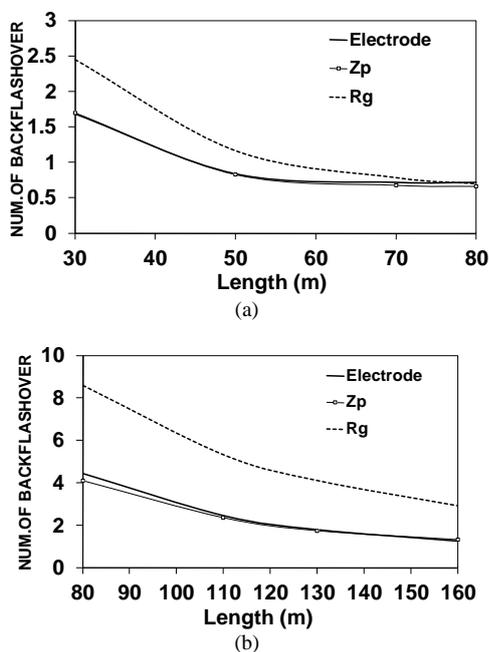
Figure 6. Backflashover outages rates (/100 km/year) calculated from different representations of the tower-footing electrodes. Soil resistivity of: (a) 1000 and (b) 4000 Ωm. [NL = 60 flashes/100 km/year]
