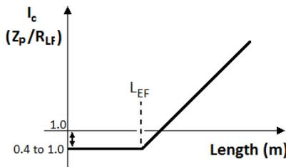
Figure 2. Typical profile of the impulse coefficient  $I_C$  as a function of the electrode length. Adapted from [1].
