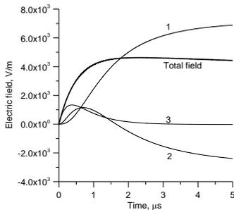
Figure 3: The total electric field at ground level at a distance of 100 m from the strike as predicted by equation 5. The three components, namely, static, induction and radiation are also shown separately by curves 1, 2 and 3 respectively. The current at the channel base is assumed to be given by  $I(t) = I_0 \{e^{-t/\tau_1} - e^{-t/\tau_2}\}$  with  $I_0 = 8.18$  kA,  $\tau_1 = 50$   $\mu$ s,  $\tau_2 = 0.5$   $\mu$ s.
