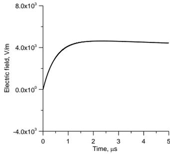
Figure 2: The electric field at ground level at a distance of 100 m from the strike as predicted by equation 1. The current at the channel base is assumed to be given by  $I(t) = I_0 \{e^{-t/\tau_1} - e^{-t/\tau_2}\}$  with  $I_0 = 8.18$  kA,  $\tau_1 = 50$   $\mu$ s,  $\tau_2 = 0.5$   $\mu$ s.
