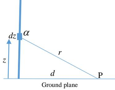
Figure 1: Geometry relevant to the calculation of electric field generated by a lightning channel located over a perfectly conducting ground plane. The channel is located along the  $z$ -axis.
