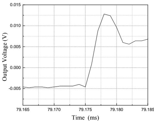
Fig.12 Detailed waveform of a voltage jump during one charging process
