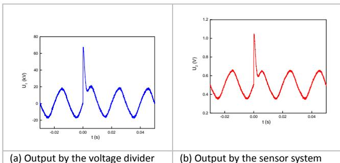
Fig.4 Waveforms of operating overvoltage experiment
