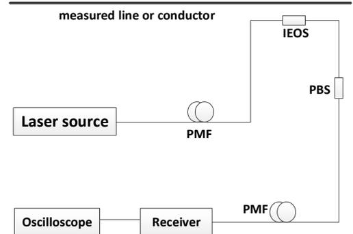
Fig. 2. The structure of the measuring system
