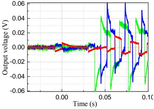
Fig.10 Waveform of the transient voltage after decoupling (Blue-A phase; Red-B phase; Green-C phase)
