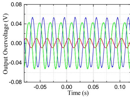
Fig.11 Waveform of power frequency voltage after decoupling (Blue-A phase; Red-B phase; Green-C phase)
