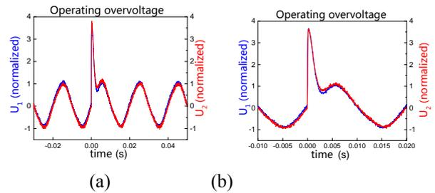
Fig.5 Normalized waveforms of operating overvoltage experiment
