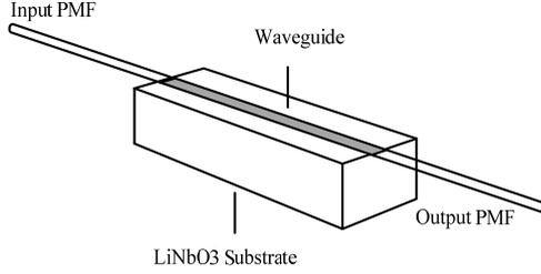
Fig 1 The structure of IEOS
