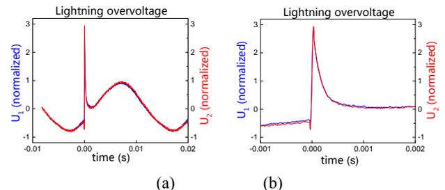
Fig.6 Normalized waveforms of lightning overvoltage experiment
