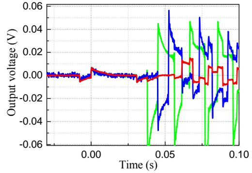
Fig.8 Waveform of the transient voltage (Blue-phase A; Red-phase B; Green-phase C)
