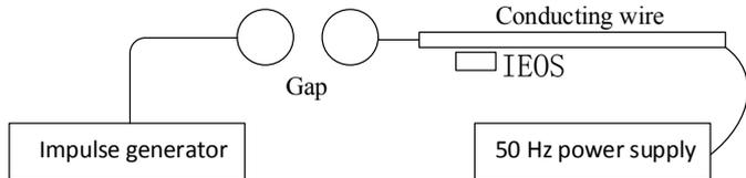
Fig 3. The configuration of the simulation experiment
