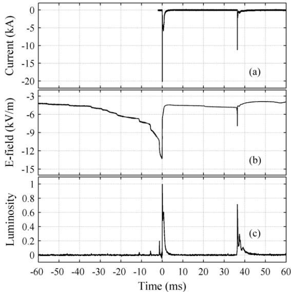
Figure 4. Recorded waveforms of (a) Current, (b) electric field measured at the secondary area (700 m) and (c) luminosity variation in relative units of Flash 17 (February 25<sup>th</sup>, 2015)
