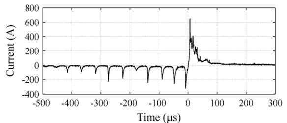
Figure 3. Waveform of an unconnected upward leader recorded at MCS on April 13<sup>th</sup>, 2014. Adapted from [6]
