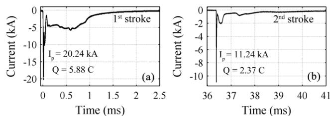
Figure 5. Current waveforms of (a) first and (b) second stroke of Flash 17
