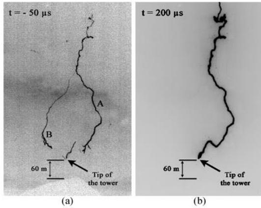
Figure 7. Frames acquired (a) just before and approximately (b) 200  $\mu$ s after the attachment of the first stroke of Flash 17 (exposure time = 50  $\mu$ s, 20,000 FPS)
