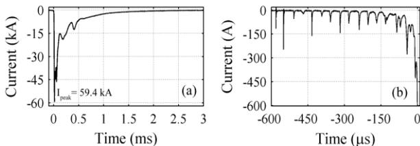
Figure 2. Current of a negative downward lightning recorded at MCS on April 13<sup>th</sup>, 2014, during (a) the return stroke process and (b) the early phase. Adapted from [6]
