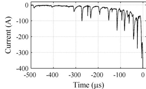
Figure 6. Initial stage of the current of the first stroke of Flash 17
