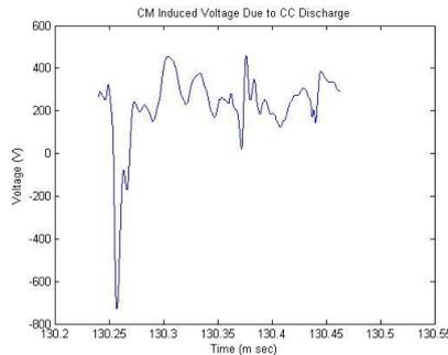
Fig. 01: (c), Pulse burst stoke V peak-peak 1056 V, CM induced voltage due to CC discharge. Incident energy of 7.30 J in 222.69 µs.
