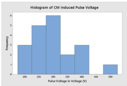
Figure 03: (a) Histogram of the CM induced peak to peak voltage on LVPI due to unipolar type pulses. Maximum, minimum and mean values of peak to peak voltages are 405 V, 181 V and 302.8 V respectively.
