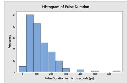
Figure 9: (b) Histogram of the total pulse duration of unipolar type induced voltages. Maximum, minimum and mean values of pulse durations are 626.3  $\mu$ s, 10.69  $\mu$ s and 121.8  $\mu$ s respectively.
