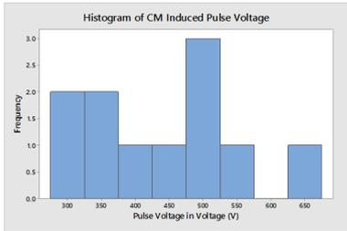
Figure 07: (a) Histogram of the CM induced peak to peak voltage on LVPI due to unipolar type pulses. Maximum, minimum and mean values of peak to peak voltages 662 V, 29 V and 449.6 V respectively.
