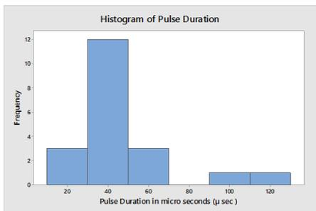
Figure 03 (b) Histogram of the total pulse duration of unipolar type induced voltages. Maximum, minimum and mean values of pulse durations are 123 µs, 11.4 µs, and 44.7 µs respectively.
