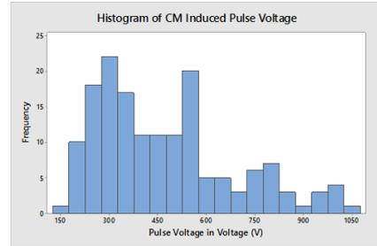
Figure 9: (a) Histogram of the CM induced peak to peak voltage on LVPI due to unipolar type pulses. Maximum, minimum and mean values of peak to peak voltages are 1056V, 171 V and 470.8 V respectively.
