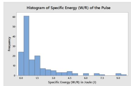
Graph 10: Histogram of the energy incident at LVPI by pulse burst type CM induced voltages. Maximum, minimum and mean values of incident energies are 9.43 J, 0.04 J and 1.46 J respectively.
