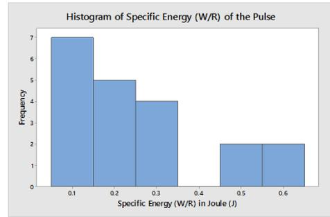
Figure 04: Histogram of the energy incident at LVPI by unipolar type CM induced voltages. Maximum, minimum and mean values of incident energies are 0.59 J, 0.06 J and 0.25 J respectively.
