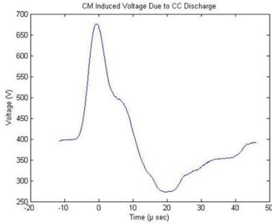
Figure 01: (a) Unipolar peak to peak Voltage 405 V CM Induced Voltage due to CC discharge. Incident energy of 0.59 J in 57.46 µs.
