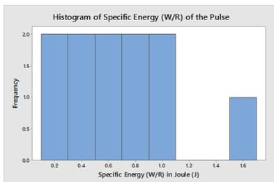
Figure 08: Histogram of the energy incident at LVPI by bipolar type CM induced voltages. Maximum, minimum and mean values of incident energies are 1.52 J, 0.22 J and 0.69 J respectively.
