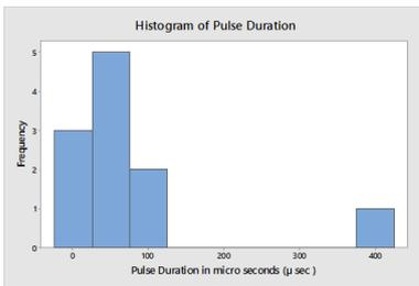
Figure 07: (b) Histogram of the total Pulse Duration of unipolar type induced voltages. Maximum, minimum and mean values of pulse durations are 401.2  $\mu$ s, 10.7  $\mu$ s and 77.5  $\mu$ s respectively.
