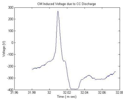
Figure 01: (b), Bipolar V peak-peak 662 V, CM induced voltage due to CC discharge. Incident energy of 0.15 J in 95.0 µs.
