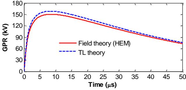
Figure 2. Grounding Potential Rise of an arrangement composed of two parallel electrodes of length (10 m each), both buried 0.5 m deep in a soil of  $3000 \Omega\text{m}$ , and set 20 m apart, subjected to an impulsive current.
