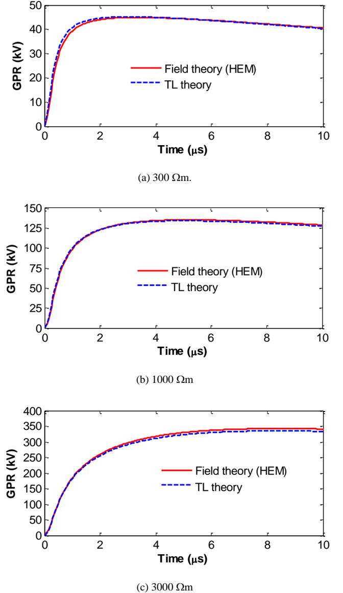
Figure 1. Grounding Potential Rise of an arrangement composed of three vertical grounding rods of 3 m forming an equilateral triangle (side = 1 m), subjected to an impulsive current.
