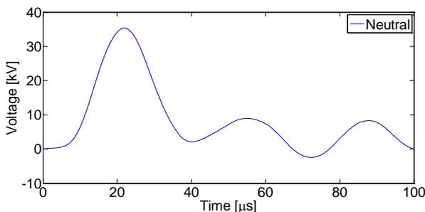
Figure 10. Voltage grounding grid in transformer at 680 node. Include phase – phase surge arrester to protect delta windings.
