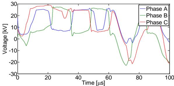
Figure 9. Voltage in phases to neutral wire substation at 680 node. None include phase – phase surge arrester to protect delta windings.
