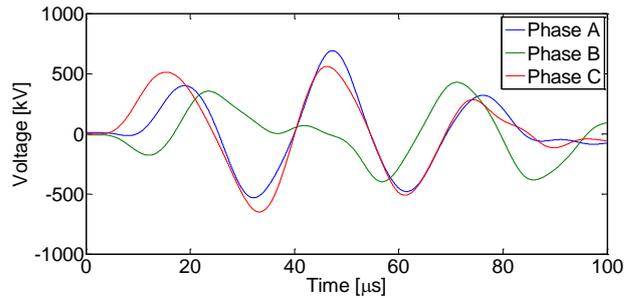
Figure 7. Voltage in phases to neutral wire substation at the node 680. Without any surge arrester to protect the windings.
