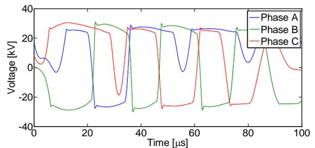
Figure 8. Voltage in phases to neutral wire substation at 680 node. A phase – phase surge arrester to protect delta windings is not included.
