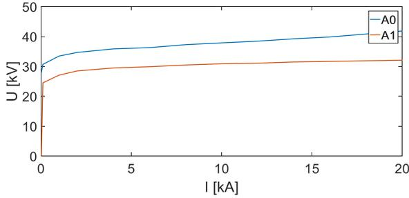
Figure 3.  $A_0$  and  $A_1$  response for the LV surge arrester implemented.
