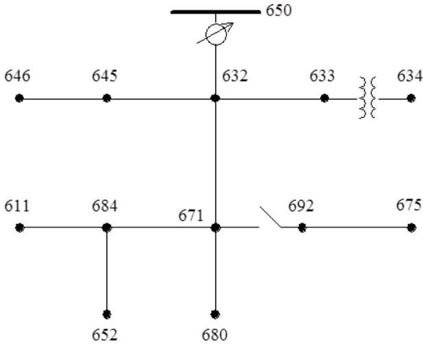
Figure 1. IEEE 13 nodes bus test feeder [13]
