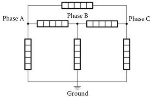
Figure 4. Phase to phase protection delta winding [9].
