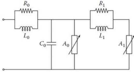
Figure 2. IEEE MO arrester model for fast front surges [20].
