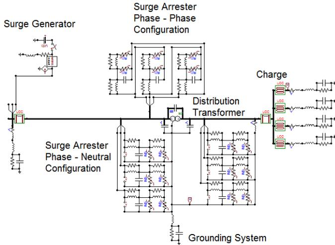
Figure 6. Simplification of IEEE 13 bus test feeder model implemented in EMTP - ATP.
