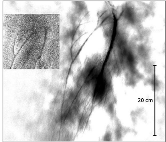
Fig. 7. Simultaneous IR image of the event recorded in Fig.6. Exposure time of the FLIR 7700M camera is 8 ms. Shown in the upper left corner is a fragment of Fig.6 depicting UPFs in the visible range. It can be seen that the contours of the brightest UPFs are similar in both images.
