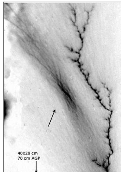
Fig. 3. Infrared image (negative) obtained with 6.7 ms exposure that shows the upper part of the upward positive (right) leader and (left) UPF, both inside the cloud; the slanted arrow points to the brightest part of UPF. The two appear to be distinct discharge processes which interact, via their streamer zones, in the lower part of the image. AGP stands for above the grounded plane.
