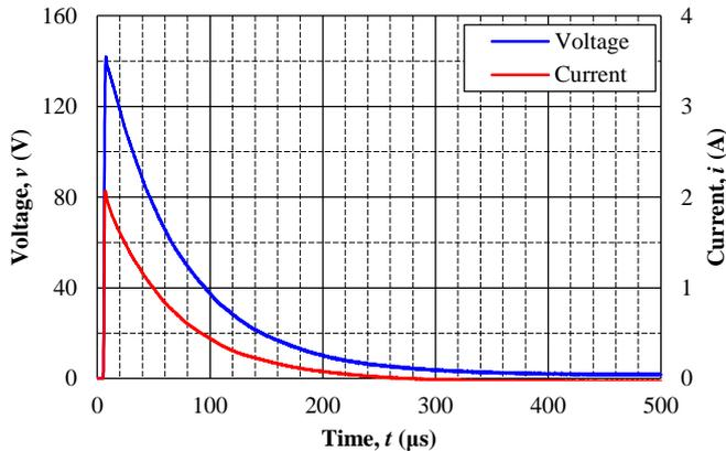
Fig 3 Transient response of the grounding rod under test
