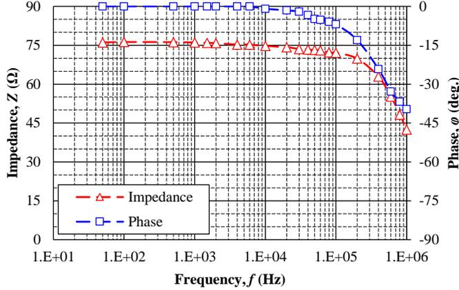
Fig 2 Amplitude and phase angle of grounding impedance of the test electrode
