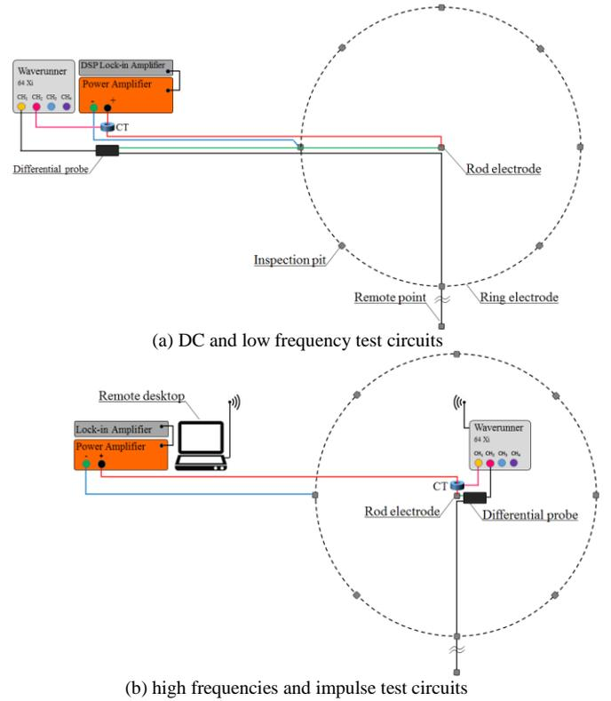
Fig. 1 Test configuration
