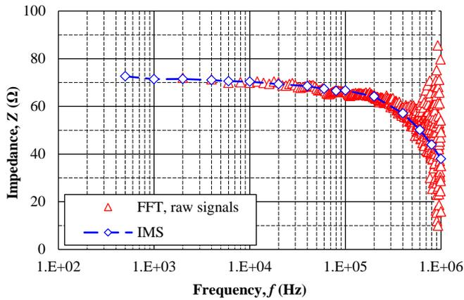
Fig 5 Frequency spectrum of grounding impedance of the test electrode obtained from the raw impulse signals
