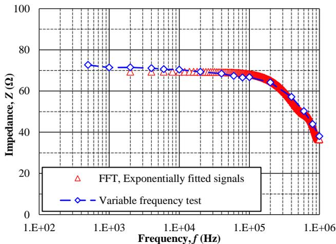
Fig 8 Frequency spectrum of grounding rod electrode impedance using direct variable frequency measurements and FFT derived spectrum with enhanced exponential fitting.
