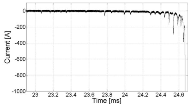
Figure 3. Unipolar pulses of current developed in response to the steps of the downward leader approaching the ground – Adapted from [11]
