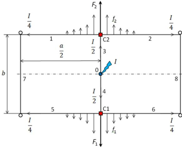
Figure 3. Sketch for the problem on ED stresses in LPS grid
