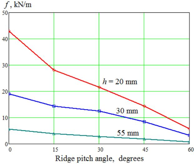
Figure 6. Forces per unit length at conductor above the ridge for various pitch angles  $\varphi$ , heights  $h$  of conductor, and 100 kA, 10/350  $\mu$ s,  $r = 4$  mm,  $d = 0.5$  mm
