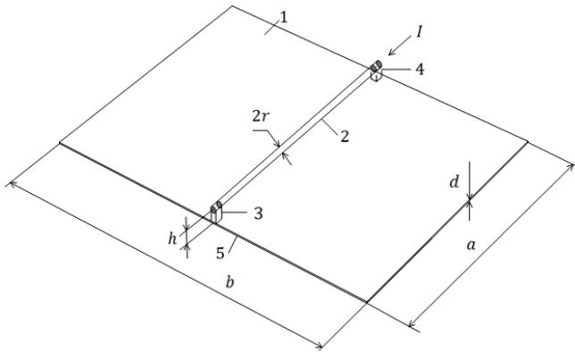
Figure 7. Model for conductor having contacts to the metal cladding: 1 – metallic sheet; 2 – conductor; 3 – holder, where conductor's end is permanently connected close to the edge 5 of 1 and earthed; 4 – holder (conductive/non-conductive) at point of current  $I$  injection
