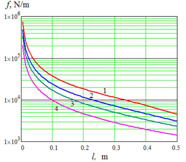
Figure 4. ED stresses  $f$  at conductors of Fig. 1b for some angles  $\varphi$  ( $l_1 = l_2 = 0.5$  m,  $I = 100$  kA): 1 to 4 –  $\varphi = 30^\circ, 45^\circ, 60^\circ, 90^\circ$ , respectively
