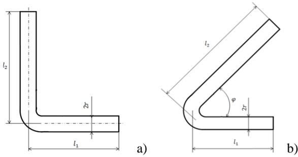
Figure 1. Bended or crossed conductors: a – angle 90°; b – other angles
