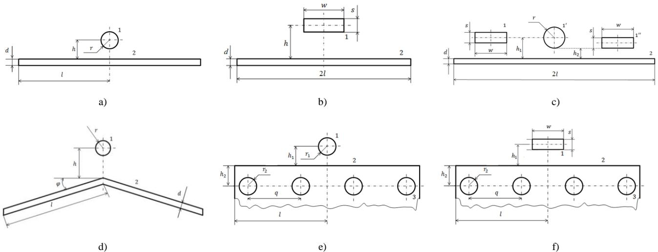
Figure 2. Model configurations of various conductors (1, 1', 1'') above metal surfaces (2), cases a, b, c, d, and reinforced concrete (2, 3), cases e, f
