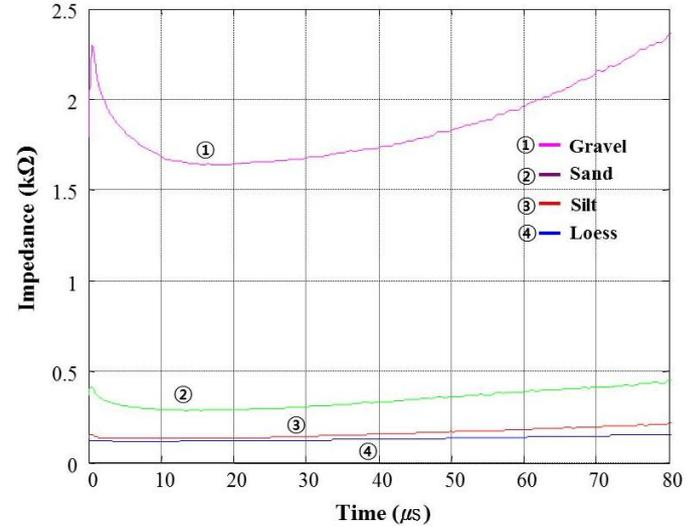
Figure 5. Examples of  $Z-t$  curves for each soil types
