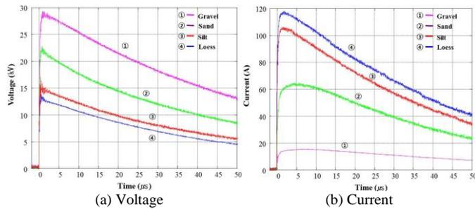
Figure 4. Impulse voltage and current waveforms when the lightning impulse voltage of 32 kV was applied between the inner and outer electrodes
