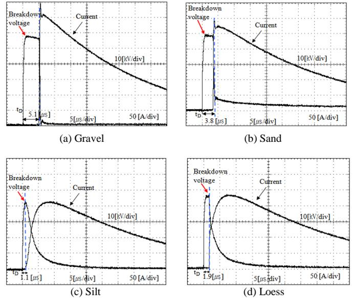
Figure 2. Typical waveforms of the breakdown voltage and current in soils
