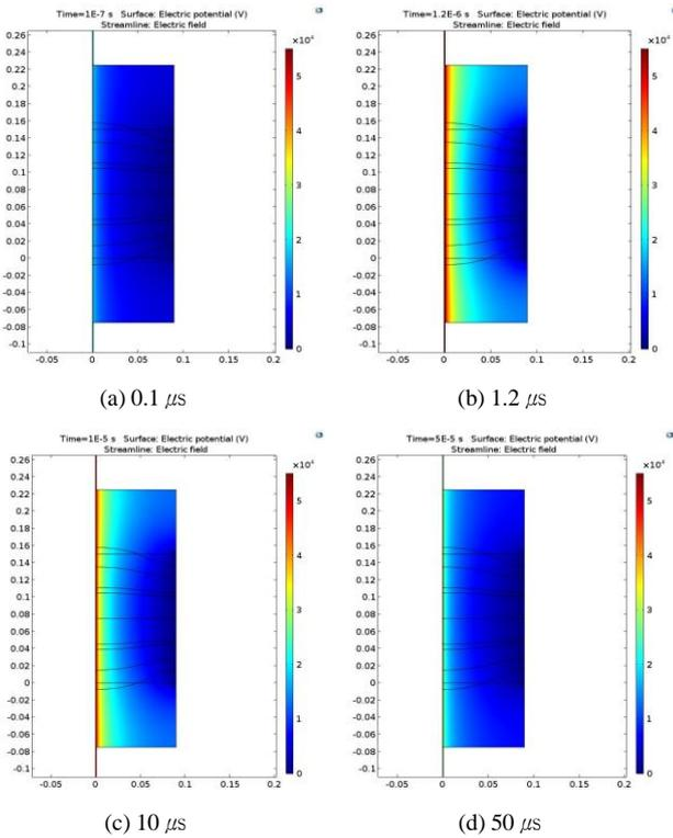
Figure 8. Electric field distribution and the streamlines formed in the vicinity of the electrode surface
