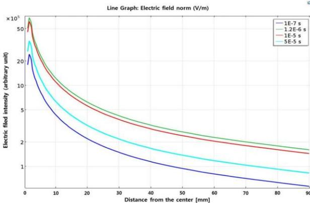
Figure 9. Electric field intensity according to the distance from the center of inner electrode stressed by the lightning impulse voltages
