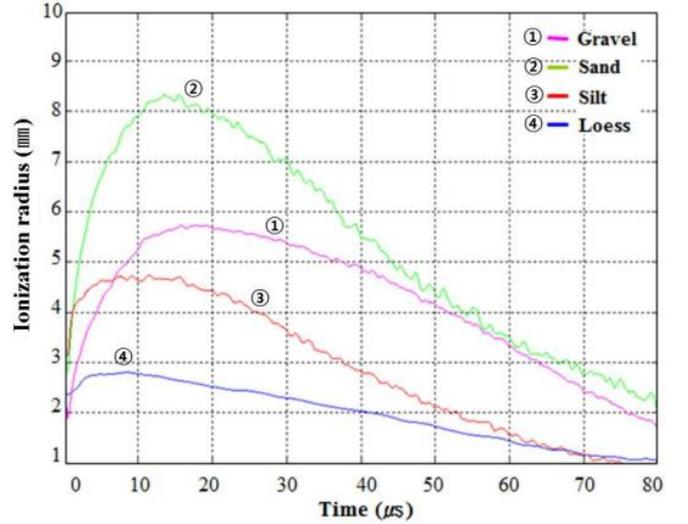
Figure 7. Equivalent ionization radius with time after the application of the lightning impulse voltage.
