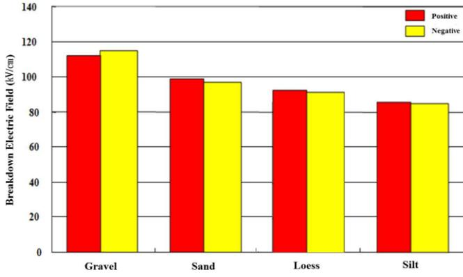
Figure 3. Electric field intensity that causes the electrical breakdown by type of soil
