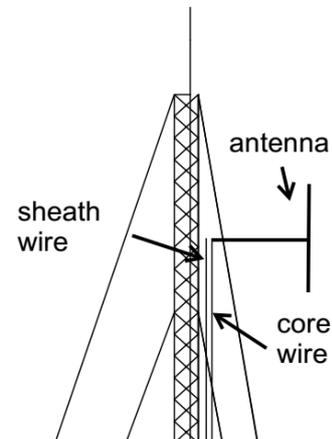
Figure 5 Close view of the tower showing conductors representing the coaxial cable and uppermost antenna
