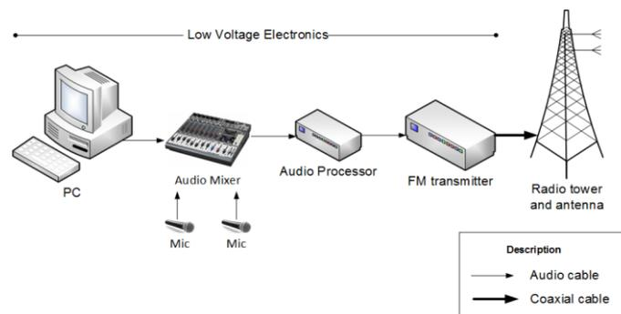
Figure 3. Local FM broadcast station diagram
