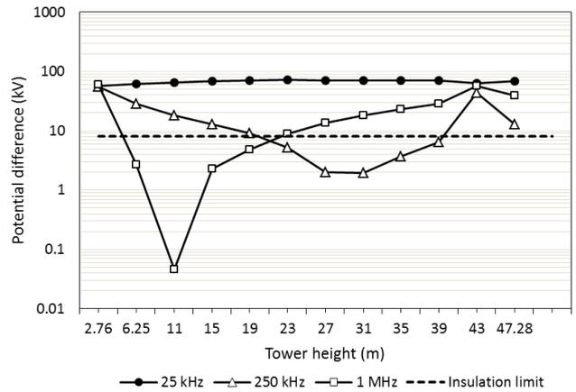
Fig. 7 Prospective potential stress on LV coaxial cable
