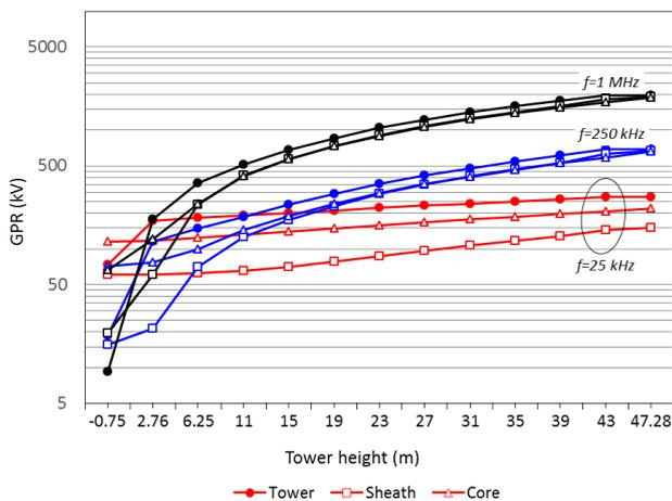
Fig. 6 Tower potentials and induced potentials along adjacent LV coaxial cable,  $\rho = 80 \Omega\text{m}$
