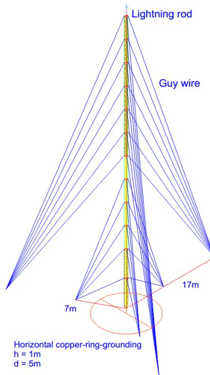
Figure 2. AutoCAD model of the three-leg guyed tower
