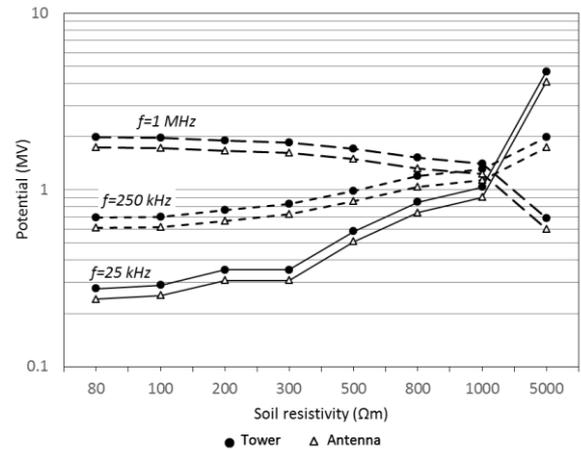
Fig. 8 Potential rise at tower and uppermost antenna
