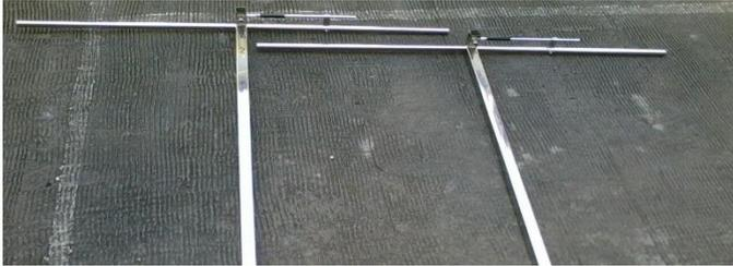
Figure 4. Vertical dipole antenna used in local FM broadcast station
