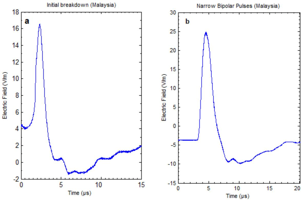
Figure 3: Similarity Characteristic between initial breakdown and narrow bipolar pulses located in Malaysia. The zero crossing time of both pulses less than 10 (μs) and have smooth rising peak from slow front to highest peak.
