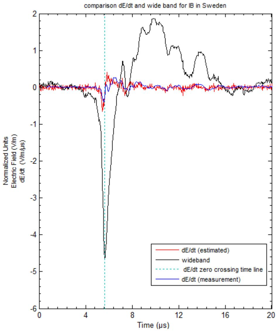
Figure 7: A comparison between Electric field in wide band, Electric field derivative (dE/dt) measurement and electric field derivative estimated by theoretically derivation for positive IB in Sweden.
