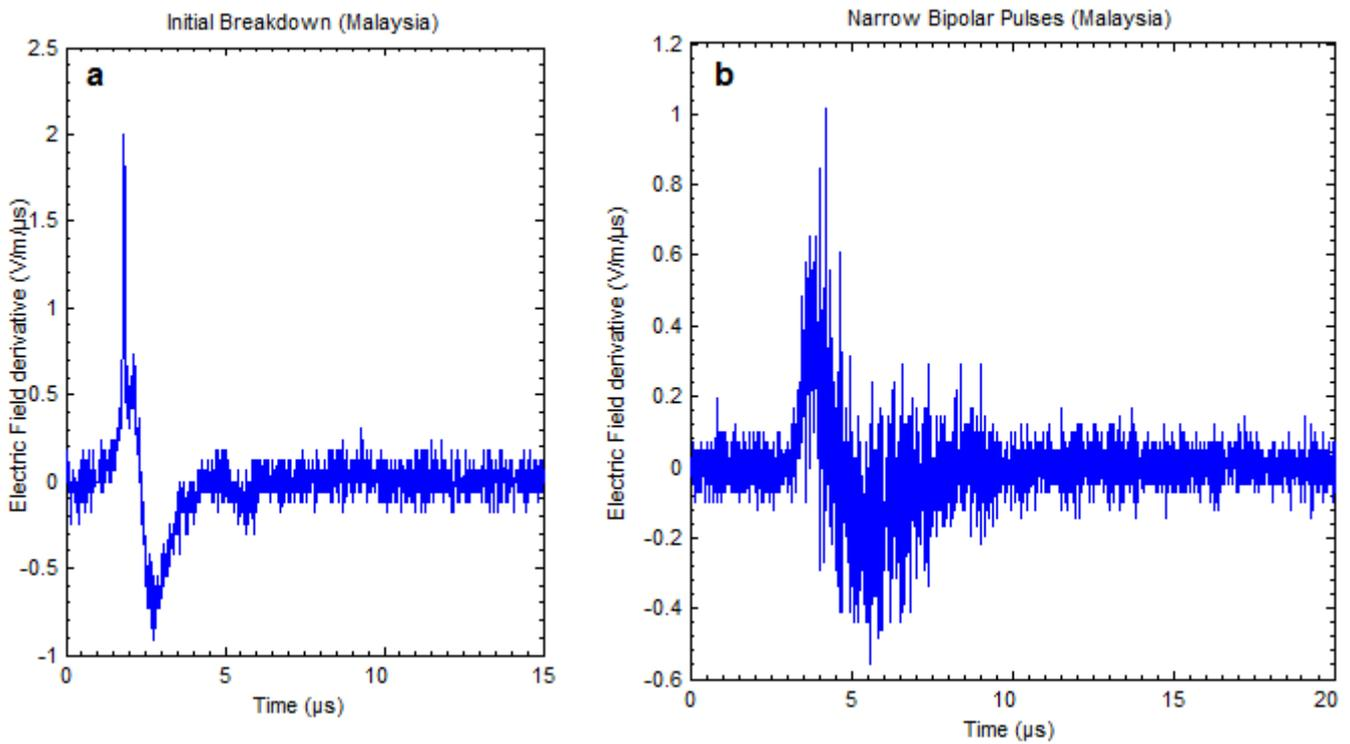
Figure 4: A comparison between initial breakdown and narrow bipolar pulses located in Malaysia based on electric field derivative (theoretically derivation).
