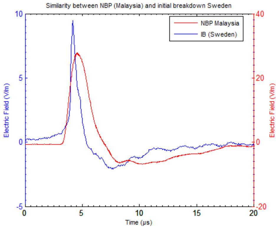
Figure 5: Similarity characteristic with smooth rising peak and zero crossing time less than 10 ( $\mu\text{s}$ ) between narrow bipolar pulses in Malaysia and initial breakdown in Sweden.
