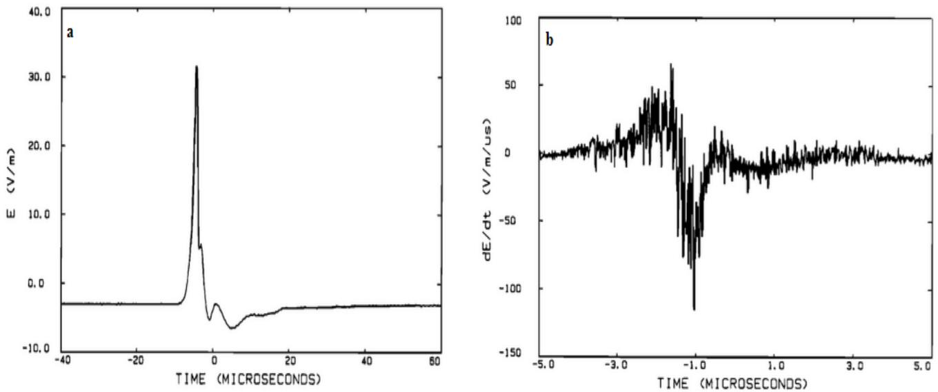
Figure 2: Narrow Bipolar Pulses adapted by Willet et. al (1989)[5] (a) Electric field in wideband measurement (b) Electric field derivative with noisy and very oscillating shape.
