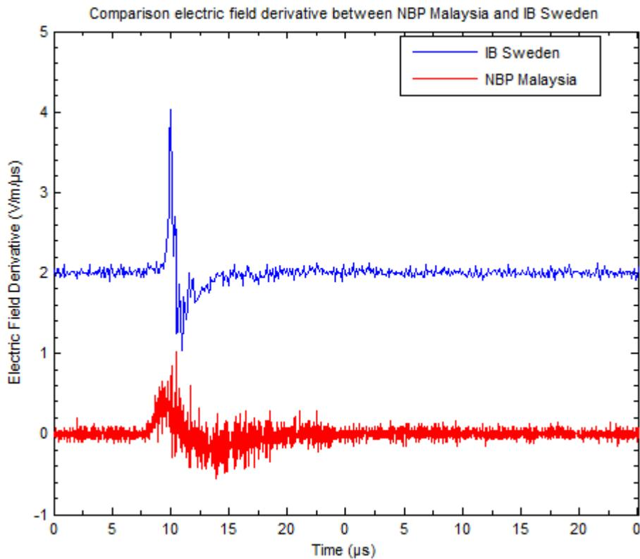
Figure 6: A comparison electric field derivative (theoretically derivation) between narrow bipolar pulses in Malaysia and initial breakdown in Sweden.
