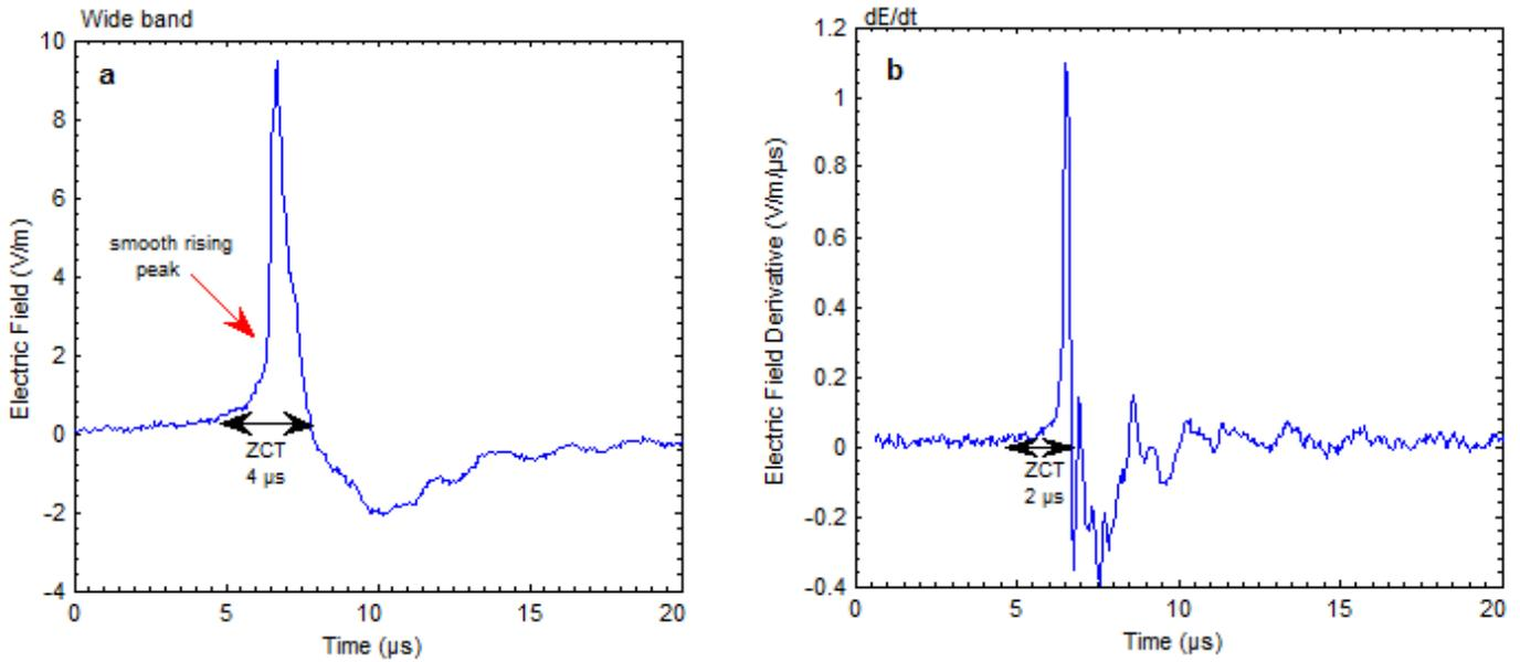
Figure 1: Initial breakdown in Sweden (a) Electric field with smooth rising peak in wideband measurement (b) Electric field derivative with less oscillating.
