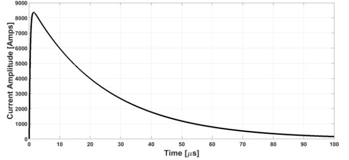
Fig. 2. Current waveform of the studied lightning signal.
