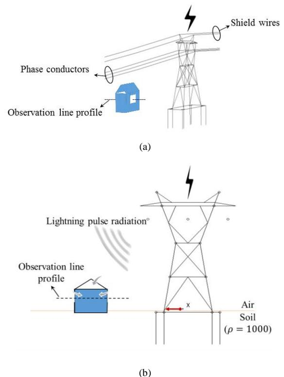
Fig. 1. Sketch of the power network hit by lightning and the shielding enclosure close to it: (a): Considering the shield wires and the phase conductors, (b): Ignoring the shield wires and the phase conductors.
