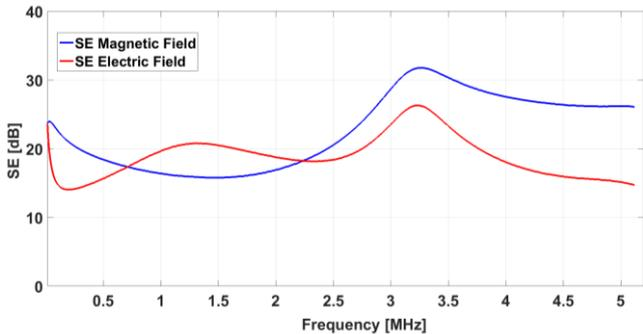
Fig. 4. Electric SE and Magnetic SE for the case ignoring the shield wires and phase conductors (Scenario 2).
