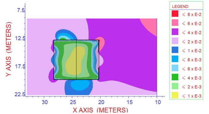
Fig. 6. The magnetic field distribution (A/m) at frequency of 3.2 MHz.
