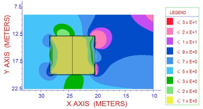
Fig. 5. The electric field distribution (V/m) at frequency of 3.2 MHz.
