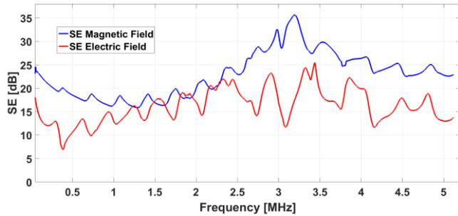
Fig. 3. Electric SE and Magnetic SE for the case considering the shield wires and phase conductors (Scenario 1).
