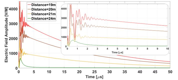
Fig. 9. Time trend of the electric field (Scenario 2).
