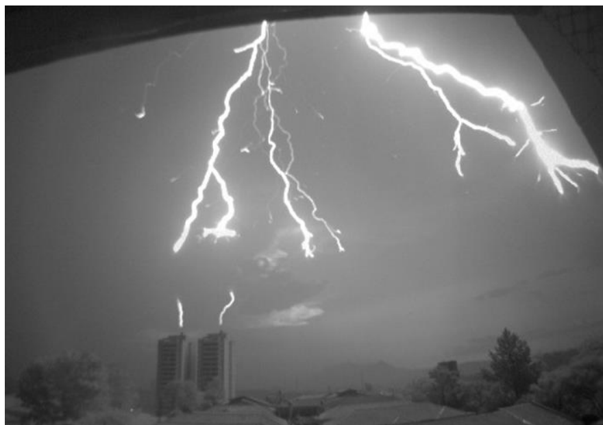
Figure 4. Image from a high-speed video of a downward leader and upward connecting leaders a few microseconds before attachment (recorded on February 9, 2014).
