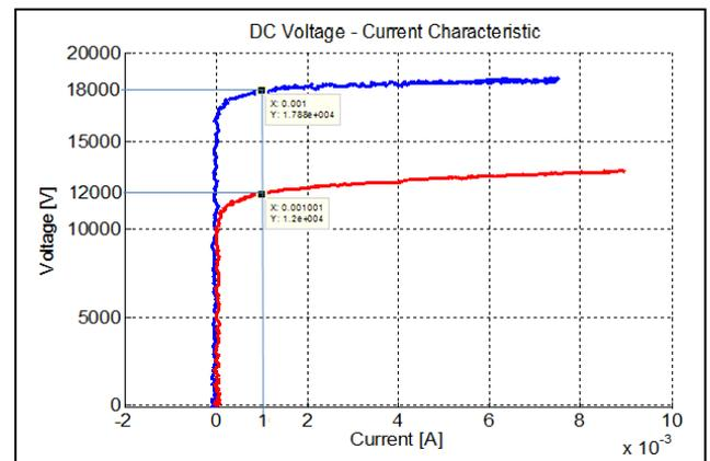
Figure 9. DC Voltage-current characteristic a) for a new surge arrester, blue line, b) for an aged surge arrester, red line. Notice the referent voltage changes at 1 mA in both blue and red characteristics.
