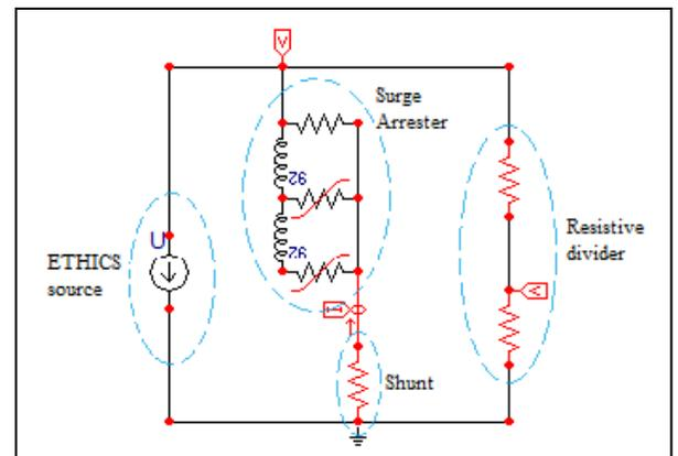
Figure 5. ETHICS DC experimental circuit. Notice the resistive divider and the shunt resistance to obtain the V-I characteristics.
