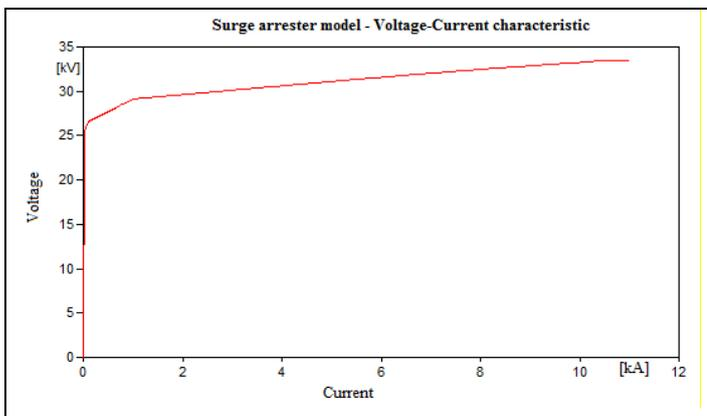
Figure 3. Surge arrester model – Voltage-current characteristic.
