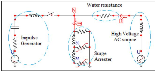
Figure 6. AC and Impulse experimental circuit to age surge arrester. Notice the water resistor used to disengage the AC source from the Current Impulse Generator.
