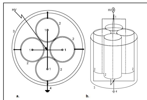
Figure 1. Extra High Impedance Current source ETHICS. a) Upper view of the four coaxial cylindrical arrangements, b) Isometric view. 1 are the corona wire electrodes, 2 are the earthed external cylindrical electrodes, 3 is a container and 4 is the earth connection [2].
