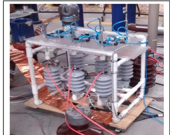
Figure 8. Isolated structure and pneumatic system
