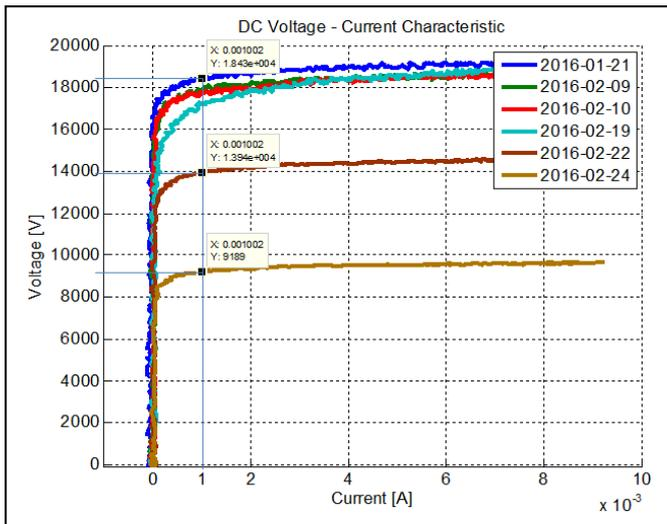
Figure 11. DC Voltage-current characteristic. S-6 sample. Notice the reference voltage changes at 1 mA for each one voltage-current characteristic.
