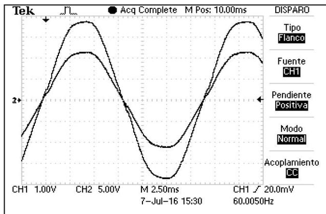
Figure 7. Voltage and current signals on water resistor
