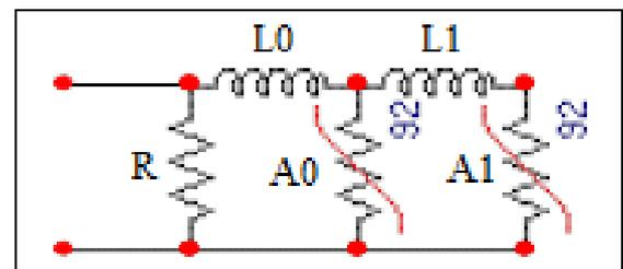
Figure 2. Surge Arrester Model according to Pinceti P. and M. Giannettoni model [7], which was used in the simulations.
