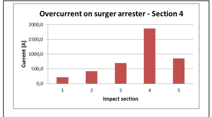
Figure 4. Calculated current in each section when the lightning current is injected in the shielding wire in section 4.
