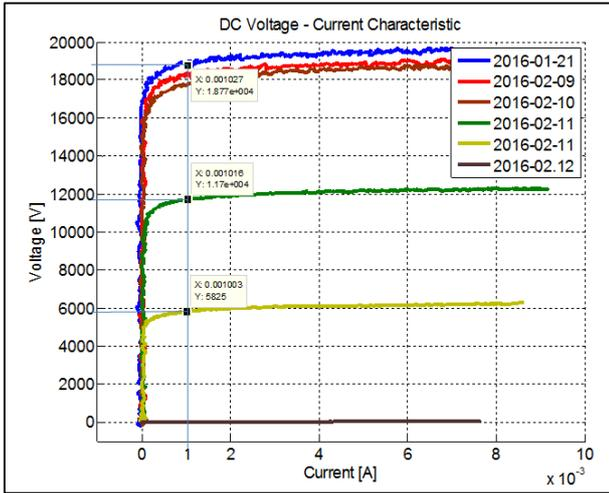
Figure 10. DC Voltage-current characteristic. S-4 sample. Notice the reference voltage changes at 1 mA for each one voltage-current characteristic.
