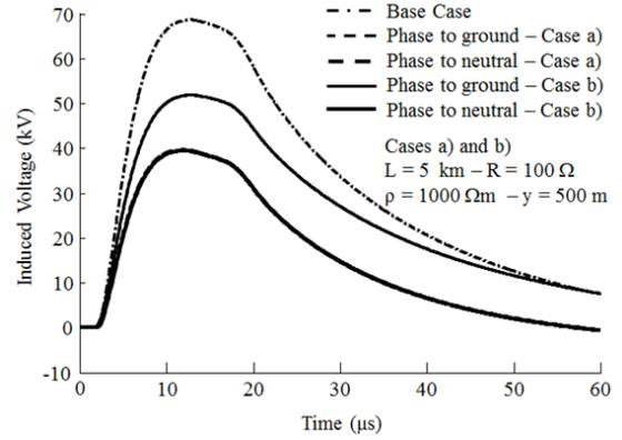
Figure 12. Phase-to-ground and phase-to-neutral LIVs for a  $1000 \Omega\text{-m}$  soil and  $y = 500$  m. Neutral conductor grounded with  $100 \Omega$  at each  $200$  m.
