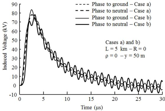
Figure 5. Phase-to-ground and phase-to-neutral LIVs for an ideal soil and  $y = 50$  m. Neutral conductor grounded with  $0 \Omega$  at each 200 m.
