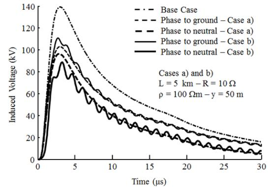
Figure 8. Phase-to-ground and phase-to-neutral LIVs for  $y = 50$  m and  $100 \Omega \cdot \text{m}$  soil. Neutral conductor grounded with  $10 \Omega$  at each 200 m.
