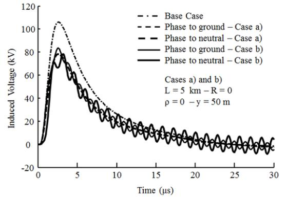
Figure 7. Phase-to-ground and phase-to-neutral LIVs for an ideal soil and  $y = 50$  m. Neutral conductor grounded with  $0 \Omega$  at each 200 m.
