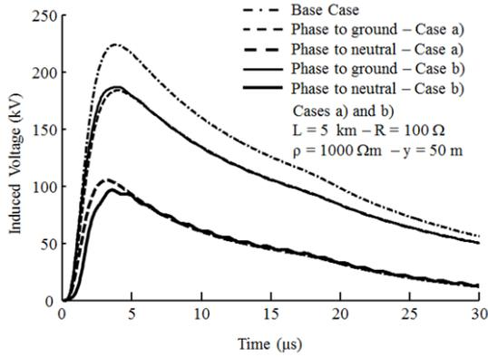
Figure 9. Phase-to-ground and phase-to-neutral LIVs for  $y = 50$  m and  $1000 \Omega\text{-m}$  soil. Neutral conductor grounded with  $100 \Omega$  at each  $200$  m.
