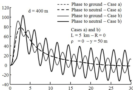
Figure 6. Phase-to-ground and phase-to-neutral LIVs for an ideal soil and  $y = 50$  m. Neutral conductor grounded with  $0 \Omega$  at each 400 m.
