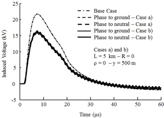
Figure 10. Phase-to-ground and phase-to-neutral LIVs for an ideal soil and  $y = 500$  m. Neutral conductor grounded with  $0 \Omega$  at each  $200$  m.
