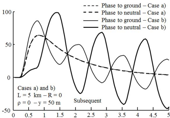
Figure 13. Phase-to-ground and phase-to-neutral LIVs for an ideal soil and  $y = 50$  m. Neutral conductor grounded with  $0 \Omega$  at each 200 m. Subsequent stroke current waveform.
