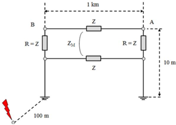
Figure 1. Line configuration used to validate the model.
