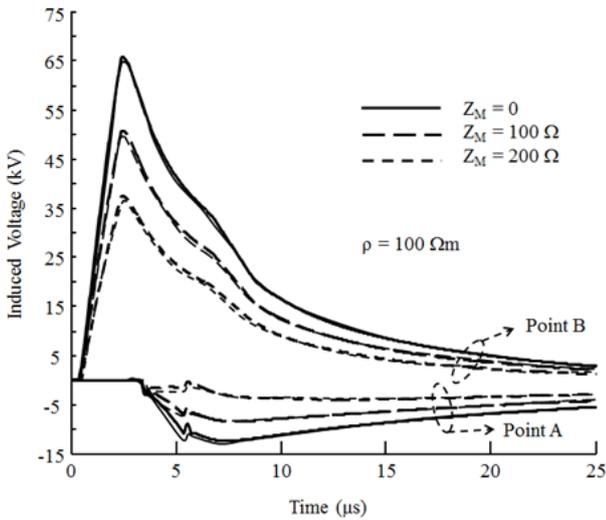
Figure 2. LIVs on both sides of the phase conductor of Fig. 1, for different values of mutual impedances between the conductors. Bold line: this paper; Thin line: results from [15].
