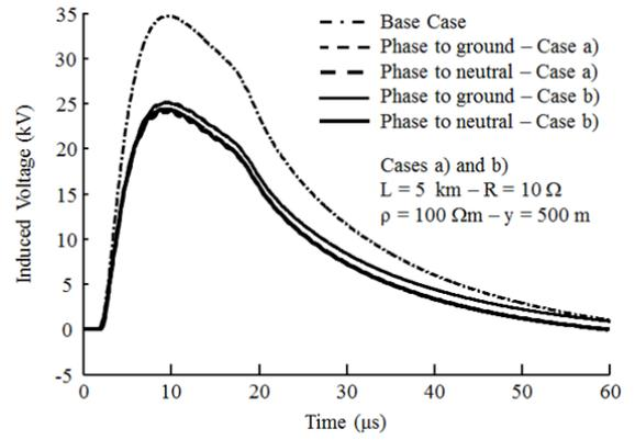
Figure 11. Phase-to-ground and phase-to-neutral LIVs for  $y = 500$  m and  $100 \Omega\text{-m}$  soil. Neutral conductor grounded with  $10 \Omega$  at each  $200$  m.
