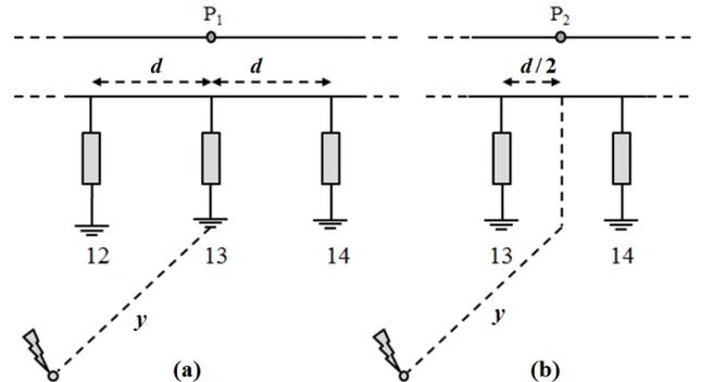
Figure 4. Stroke locations considered. (a) stroke location facing a grounding point; (b) stroke location equidistant to two consecutive grounding points.
